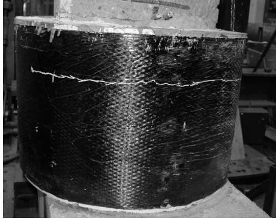
Figure 4.29 LE-R transverse CFRP crack
