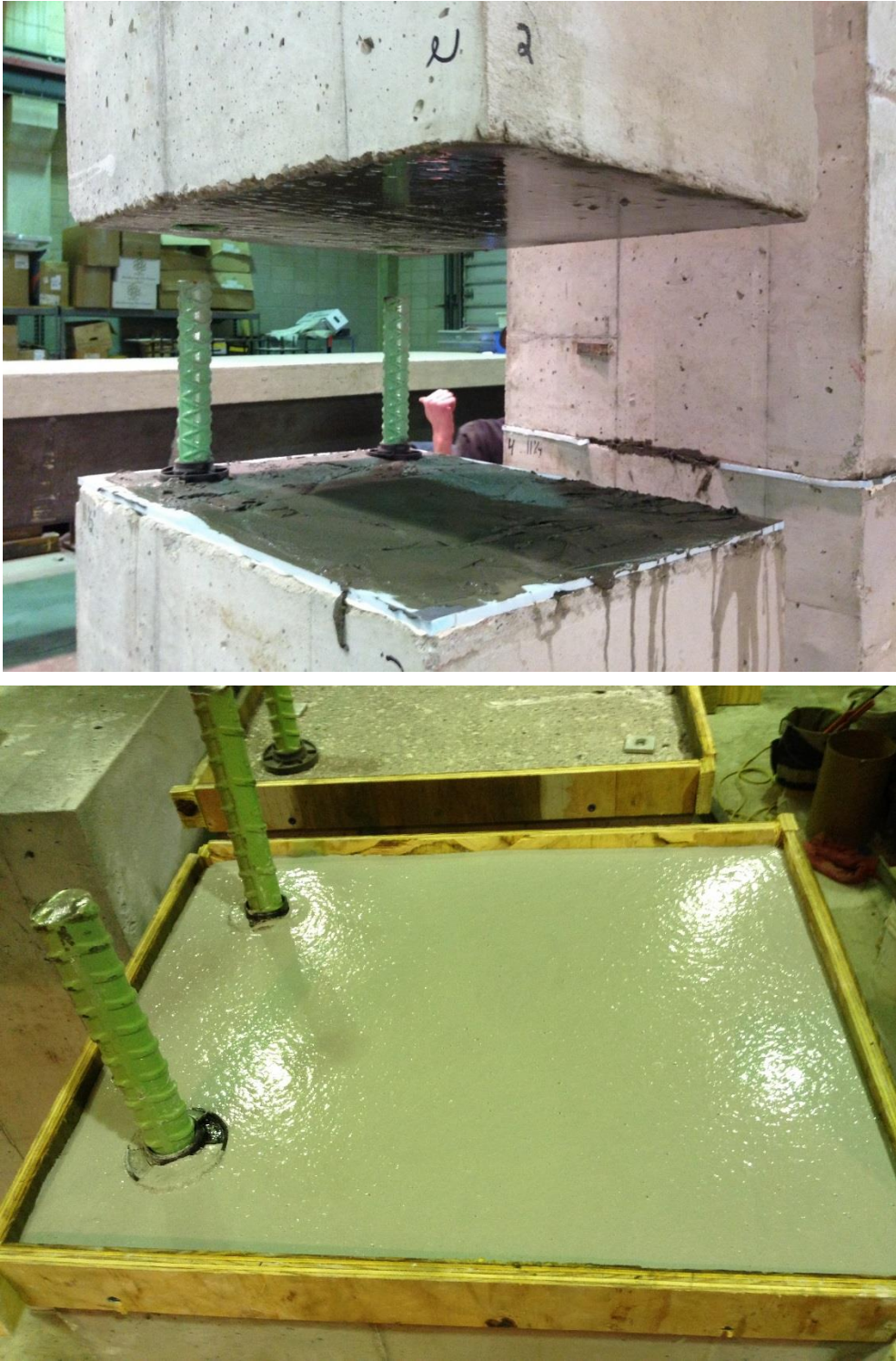
Figure 8. W. R. Meadows grout bed (top) and UHPC grout bed (bottom)
