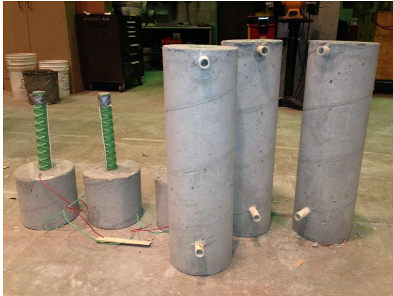
Figure 25. Small grouted coupler specimens prior to grouting
