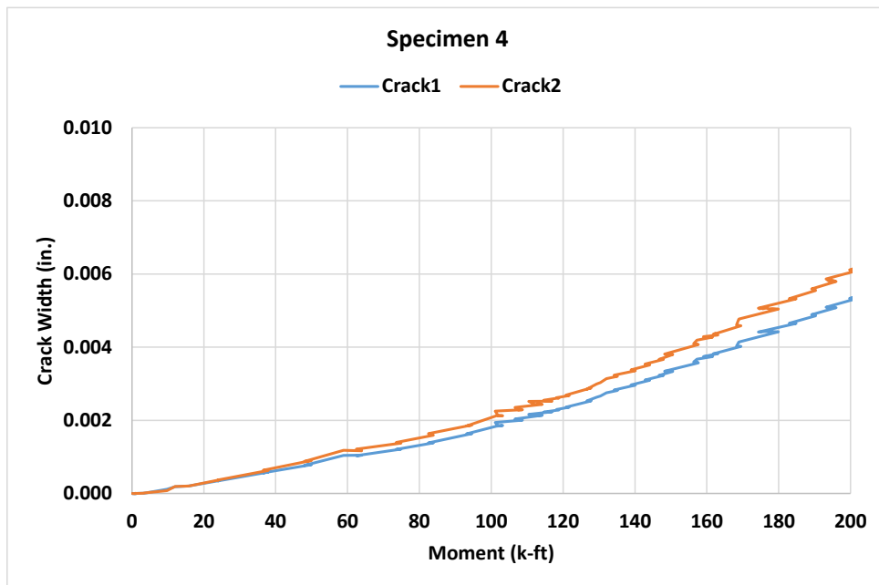
Figure 33. Typical initial crack width for specimen with axial load, Specimen 4
