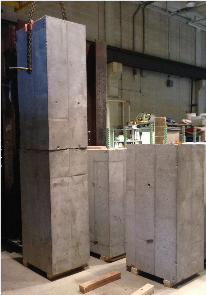
Figure 5. Dry fit of Side B on top of Side A in laboratory
