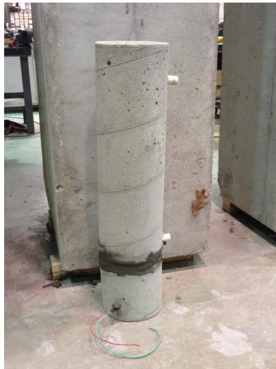
Figure 26. Small grouted coupler specimen after grouting
