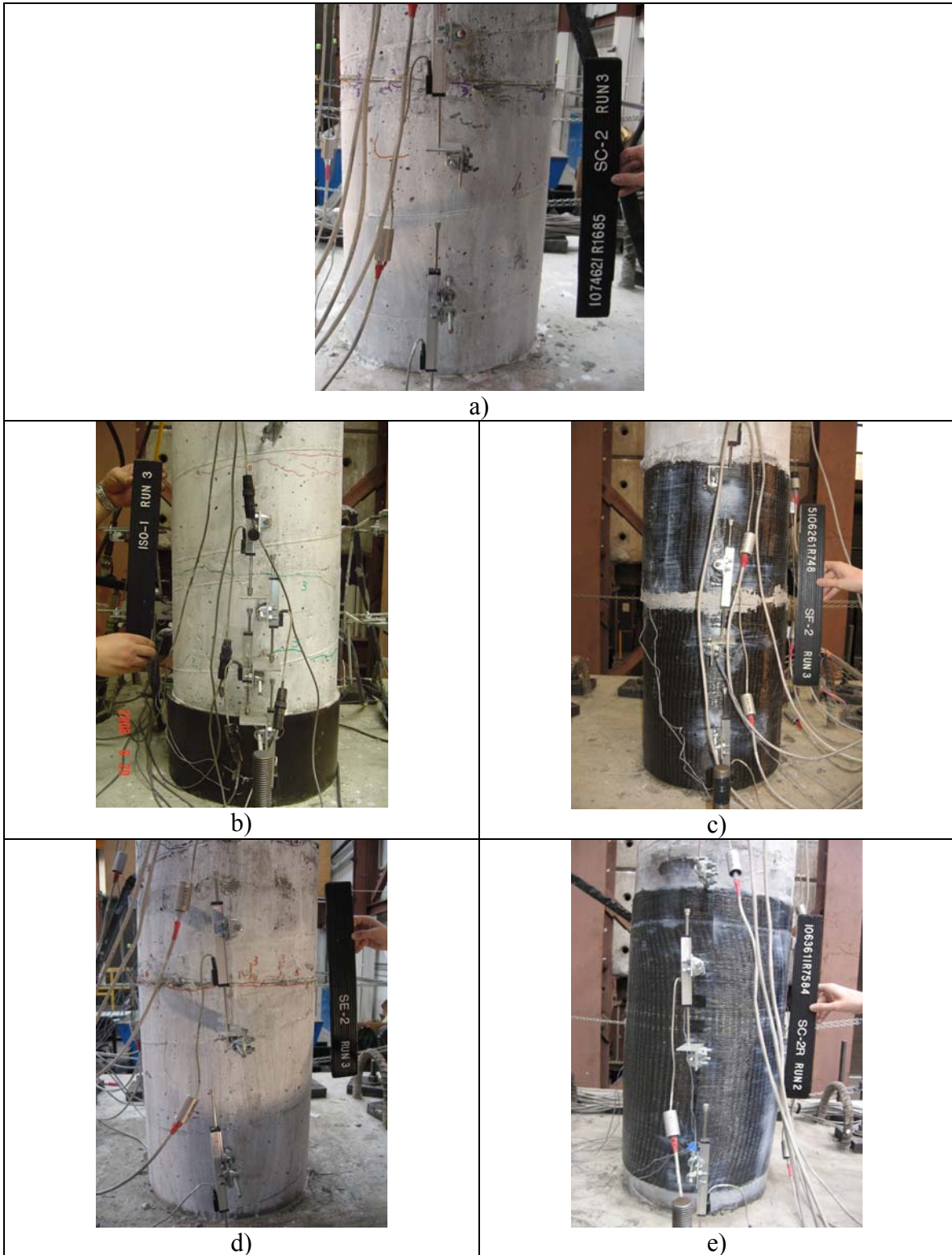
Fig. 4-1. Apparent Damage at 2% Drift for a) SC-2, b) SBR-1, c) SF-2, d) SE-2, e) SC-2R
