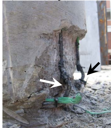
d) Two Buuckled bars, South, Run 6
