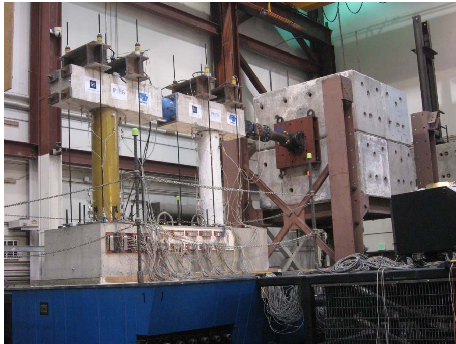
Fig. 2-86. PEFB on the Shake Table
