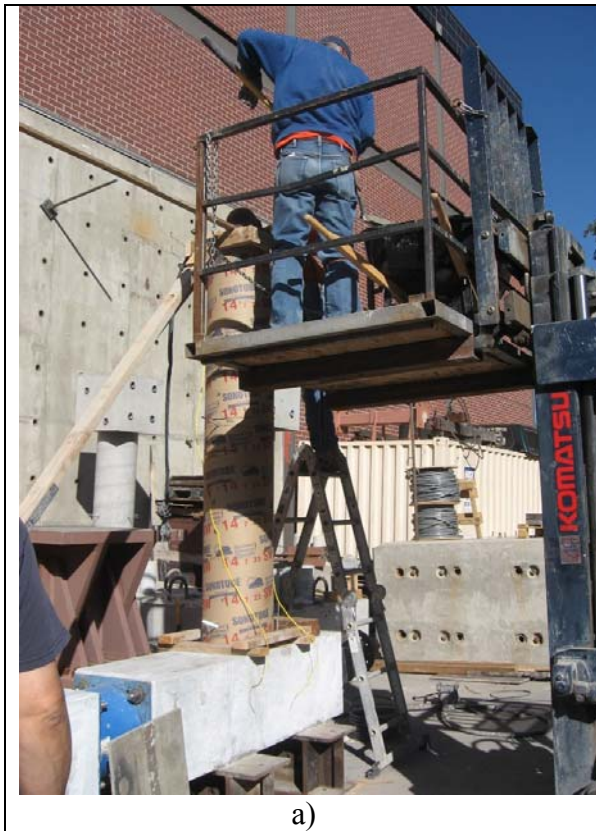
Fig. 2-73. PEFB Columns Concrete Casting, a) RC-ECC Column, b) FRP Tube
