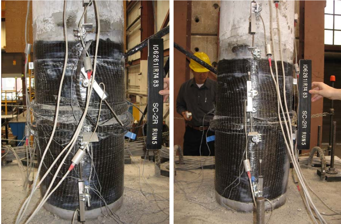
a) SC-2R Column, North, Run-5 b) SC-2R Column, South, Run-5 Fig. 3-153. Damage Progression Photographs for SC-2R Column, Bottom, Run 5
