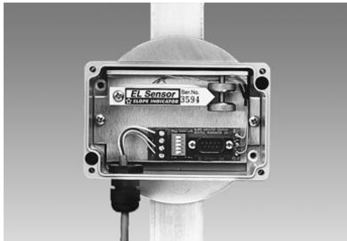
Figure 5.12 Vertical EL Tilt Sensor, interior
