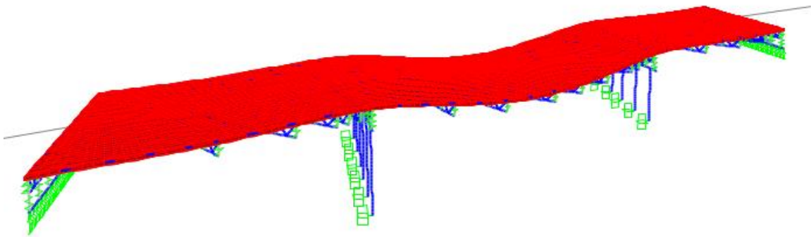
Figure 4.4 Dead load deflection of the Plattsmouth Bridge
