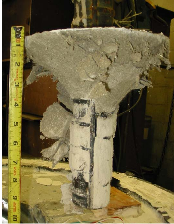
Figure 4.10: Grout cone and sheared grout: 18F04
