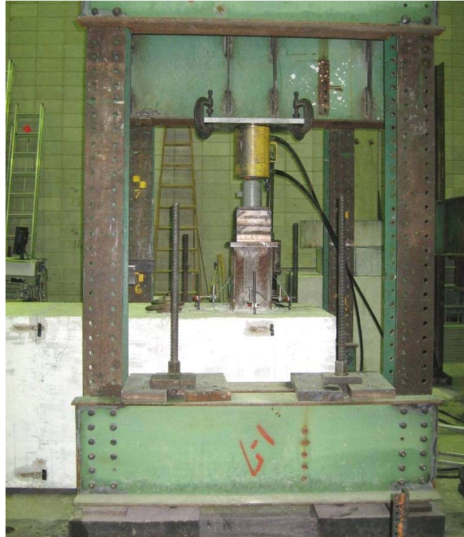
Figure 43. Double pile abutment shear Test 1
