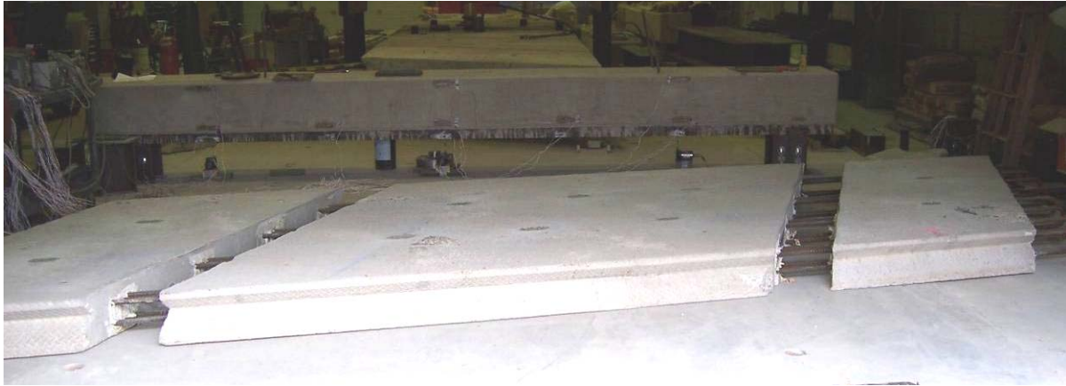
Figure 6. Boone County replacement bridge deck panel
