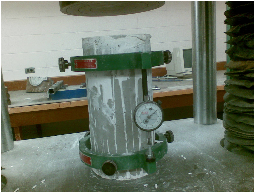
Figure A.2 Test setup for computing static modulus of elasticity of the concrete cylinders
