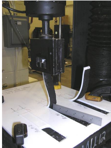
Figure 18. Bearing testing. Source: NYSDOT.
