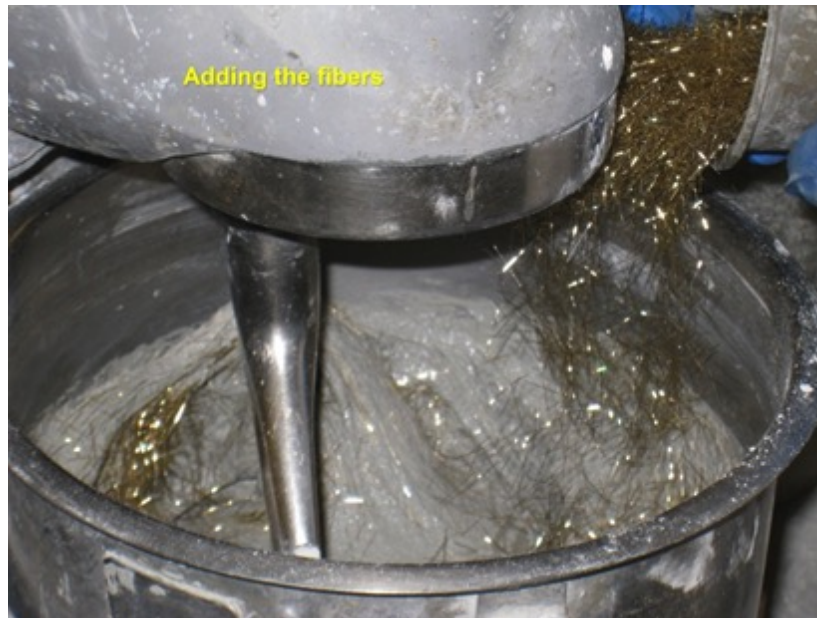
Figure 3-3 Mixing process (photos courtesy of Prof. Kay Wille)
