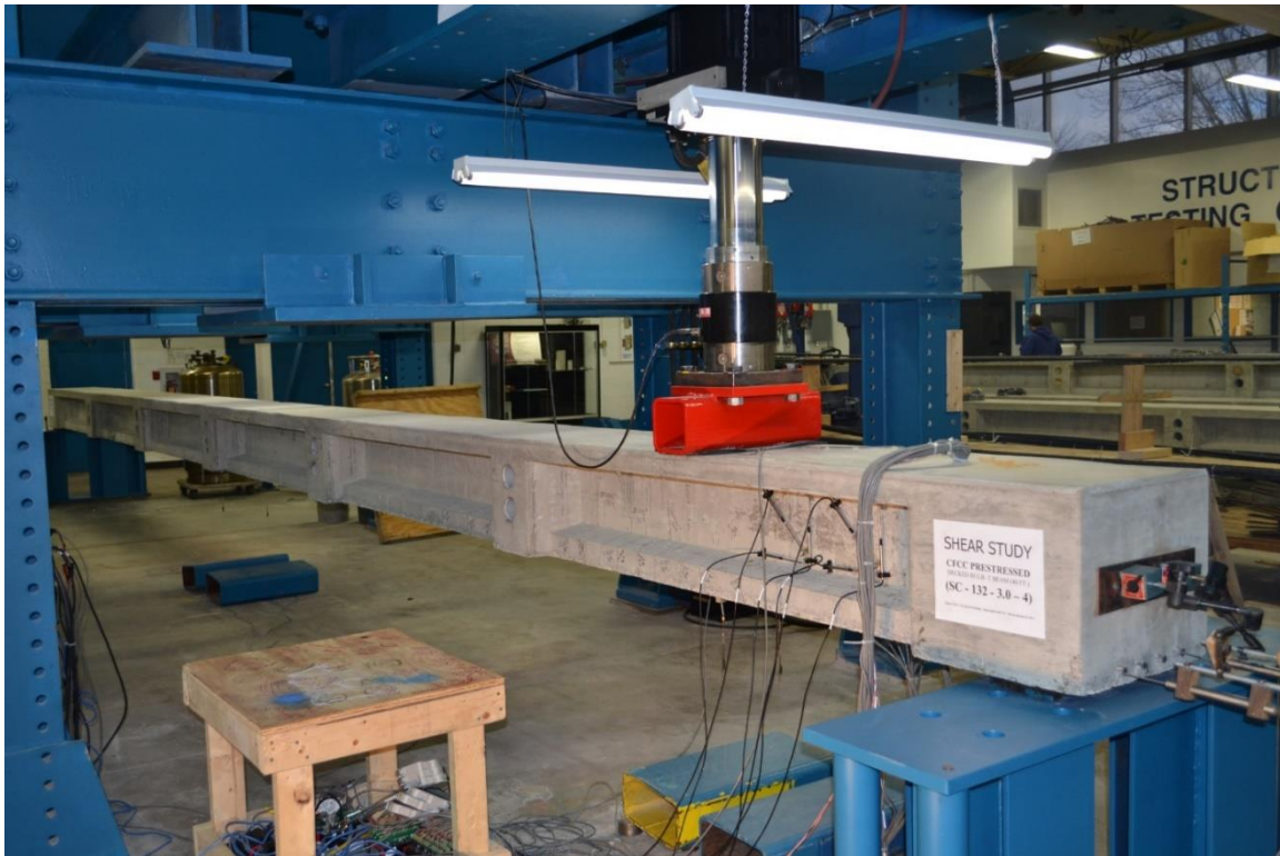
Figure 3.7-1 Test setup of Beam C-C-S-B
