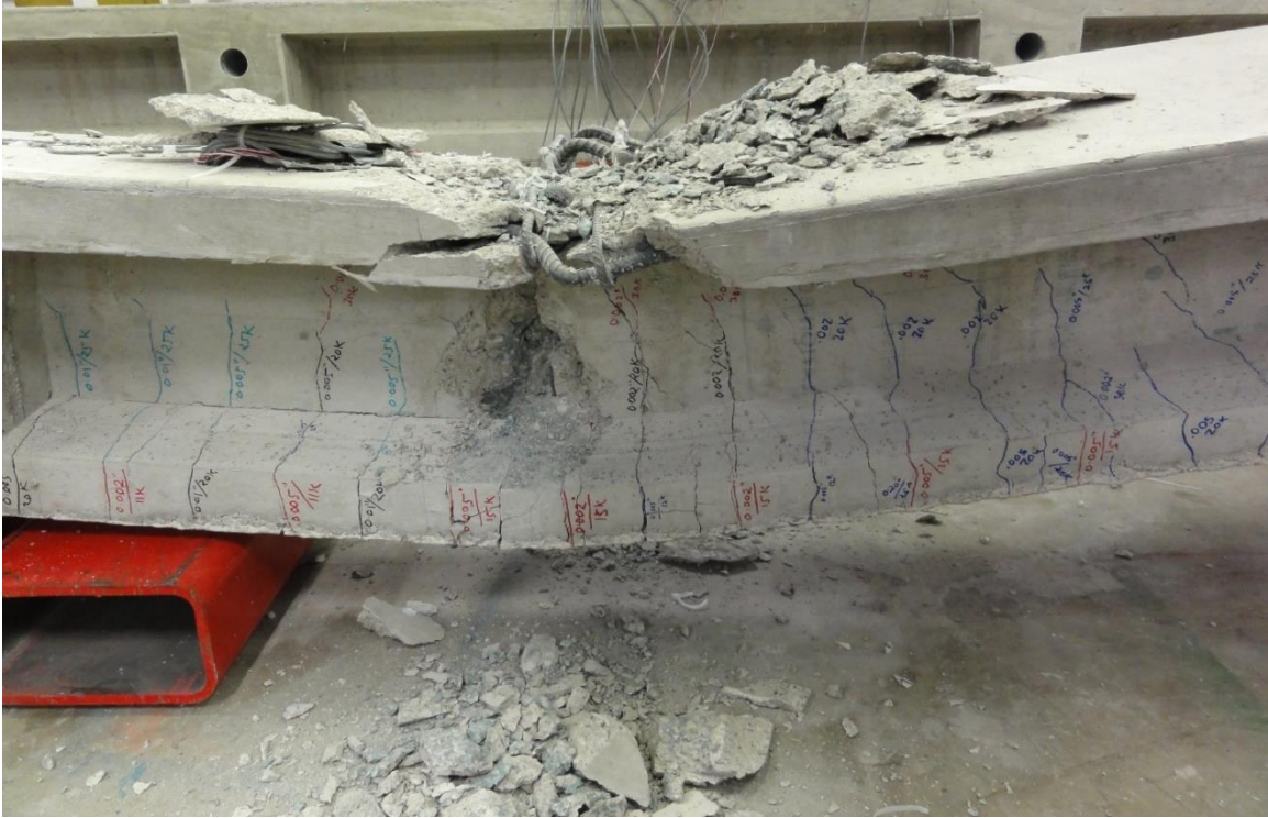
Figure 3.5-2 Failure of Beam S-S-F-U showing crushing of concrete after yield
