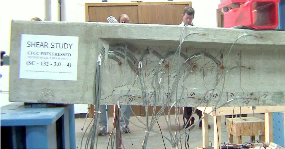
Figure 3.7-7 Development of main shear crack just before failure in Beam C-C-S-B
