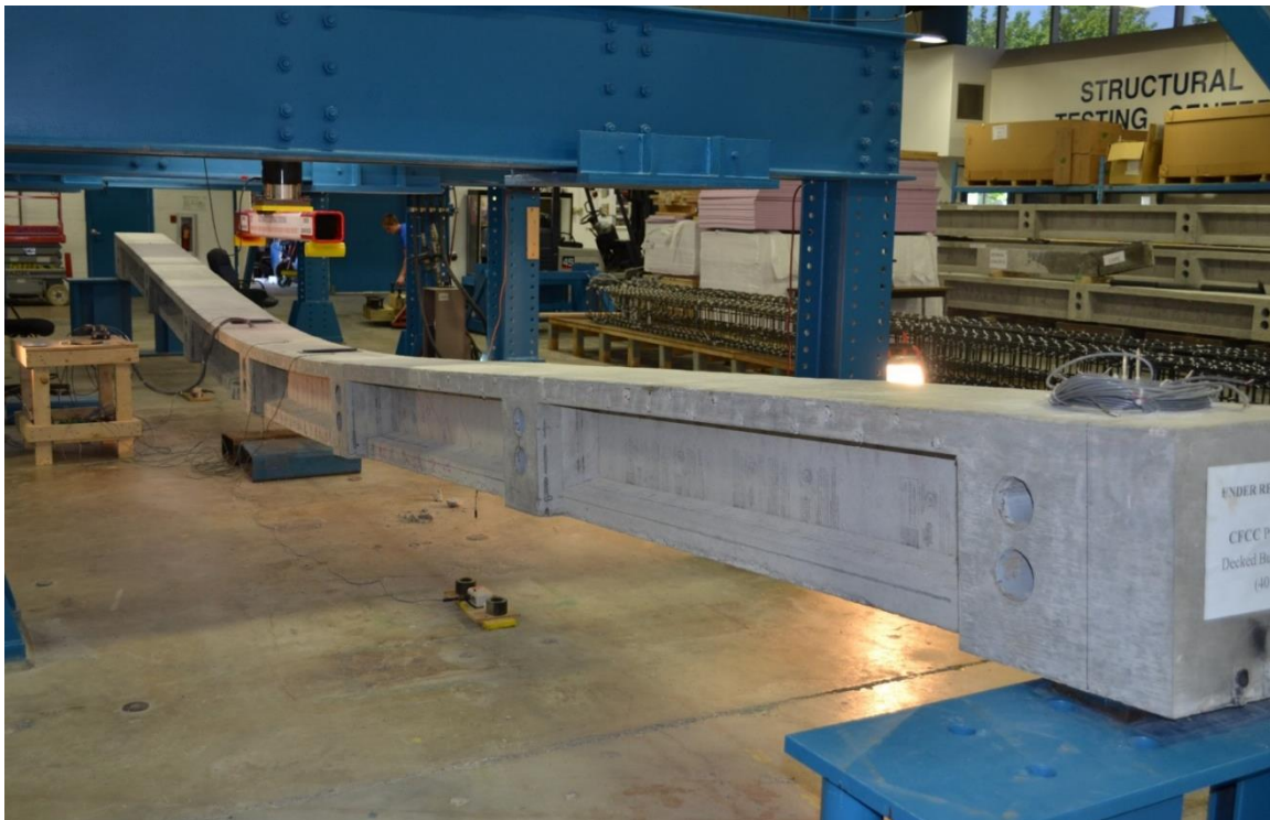
Figure 3.2-7 Beam C-S-F-U at failure
