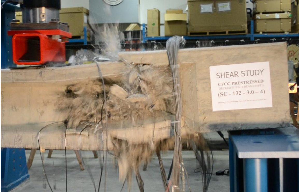
Figure 3.7-8 Explosive failure of Beam C-C-S-B
