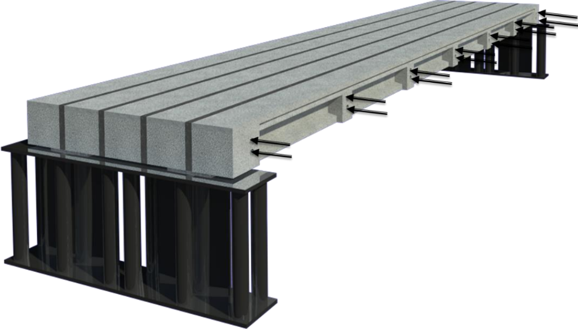
Figure 3.8-1 Schematic diagram showing the location of the transverse post-tensioning forces
