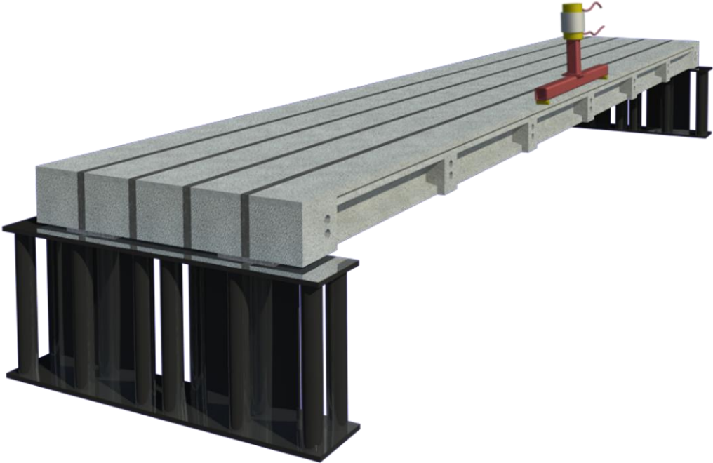
Figure 3.8-13 Schematic diagram showing testing of shear key joint
