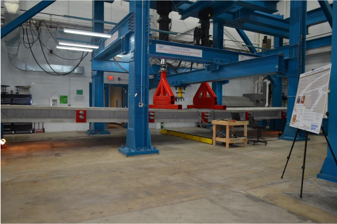
Figure 3.8-19 Load cycle test of bridge model
