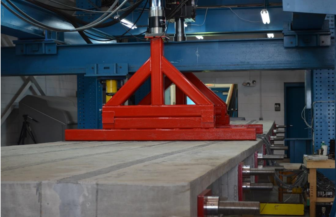
Figure 3.8-9 Four-point loading of bridge model
