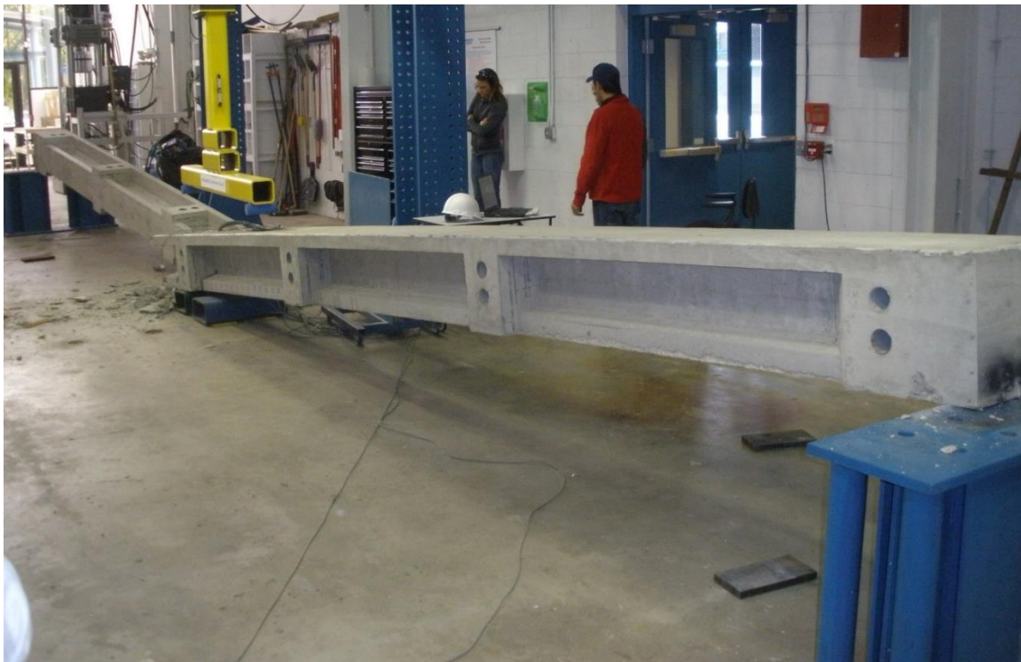
Figure 3.3-1 Balanced failure of Beam C-S-F-B
