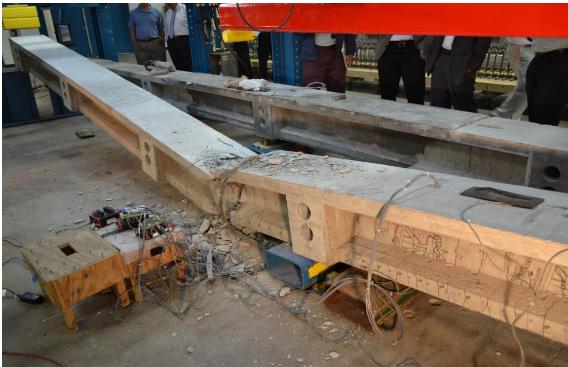
Figure 3.4-1 Beam C-S-F-O at failure
