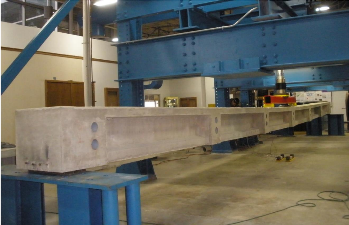
Figure 3.2-1 Typical four-point-loading test setup for control beams
