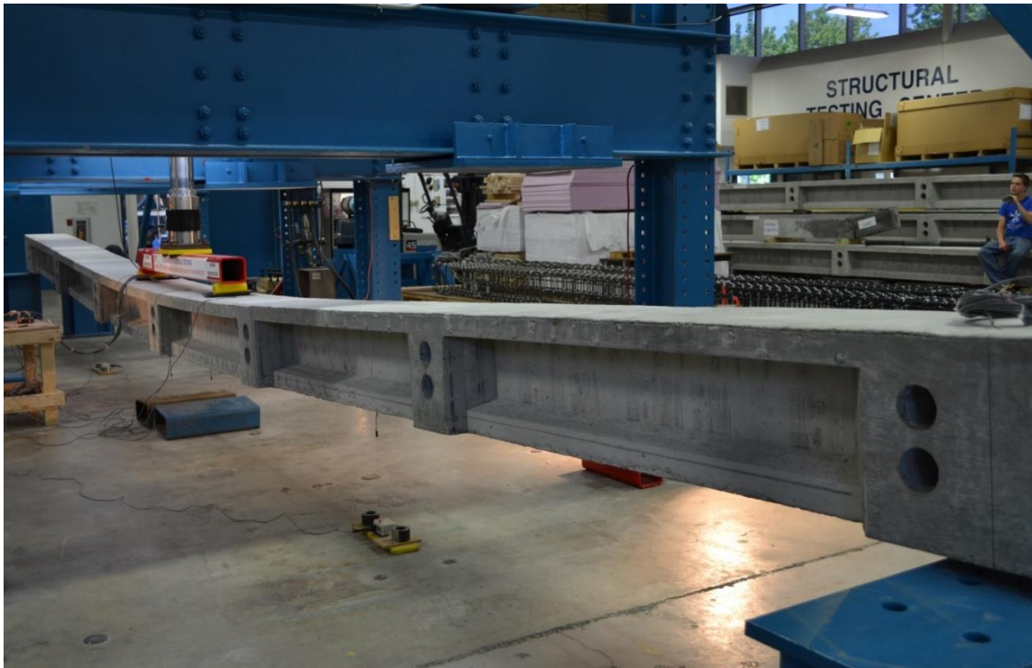
Figure 3.2-5 Deflection of Beam C-S-F-U
