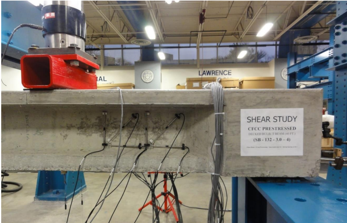
Figure 3.7-4 LVDTs at 0, 45, and 90° to evaluate shear cracking
