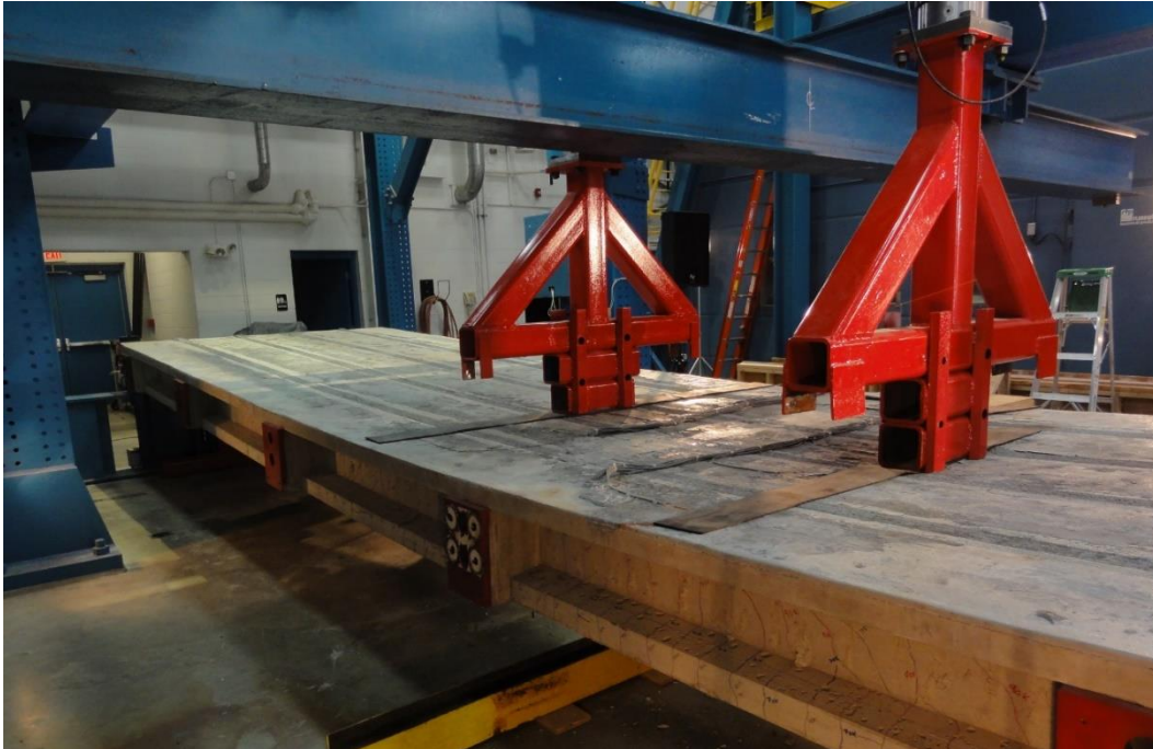
Figure 3.8-23 Four-point loading of intermediate beam at strength limit state testing
