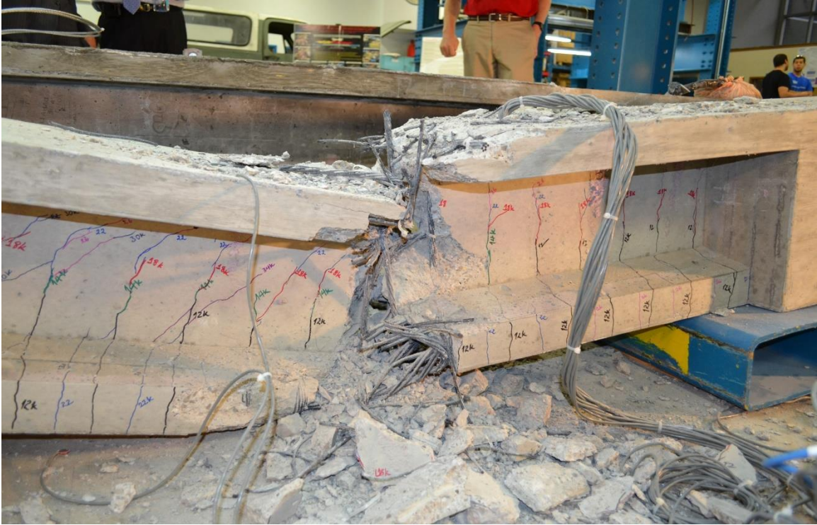
Figure 3.4-2 Compression failure followed by rupture of strands in Beam C-S-F-O
