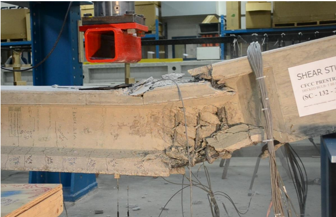
Figure 3.7-9 Beam C-C-S-B after failure
