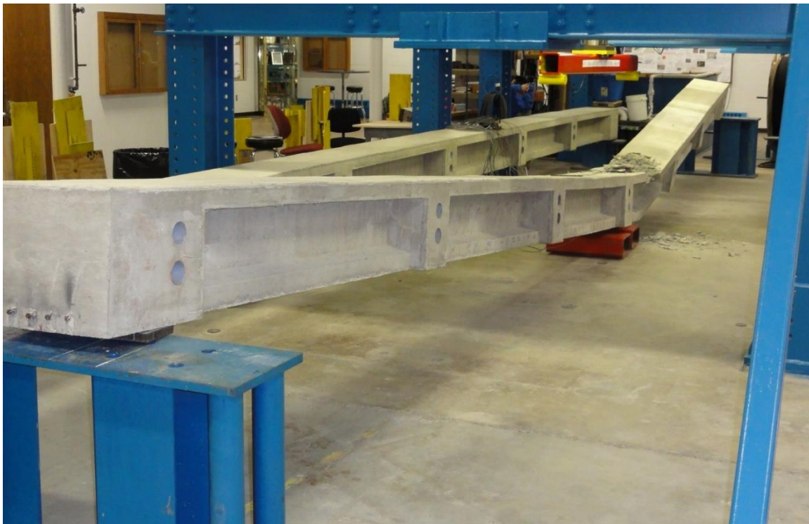
Figure 3.5-1 Flexural failure of Beam S-S-F-U
