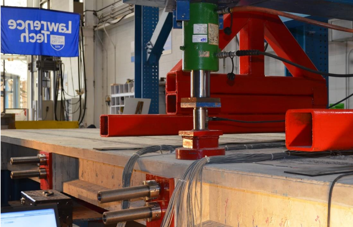
Figure 3.8-3 Service limit state testing of the bridge model
