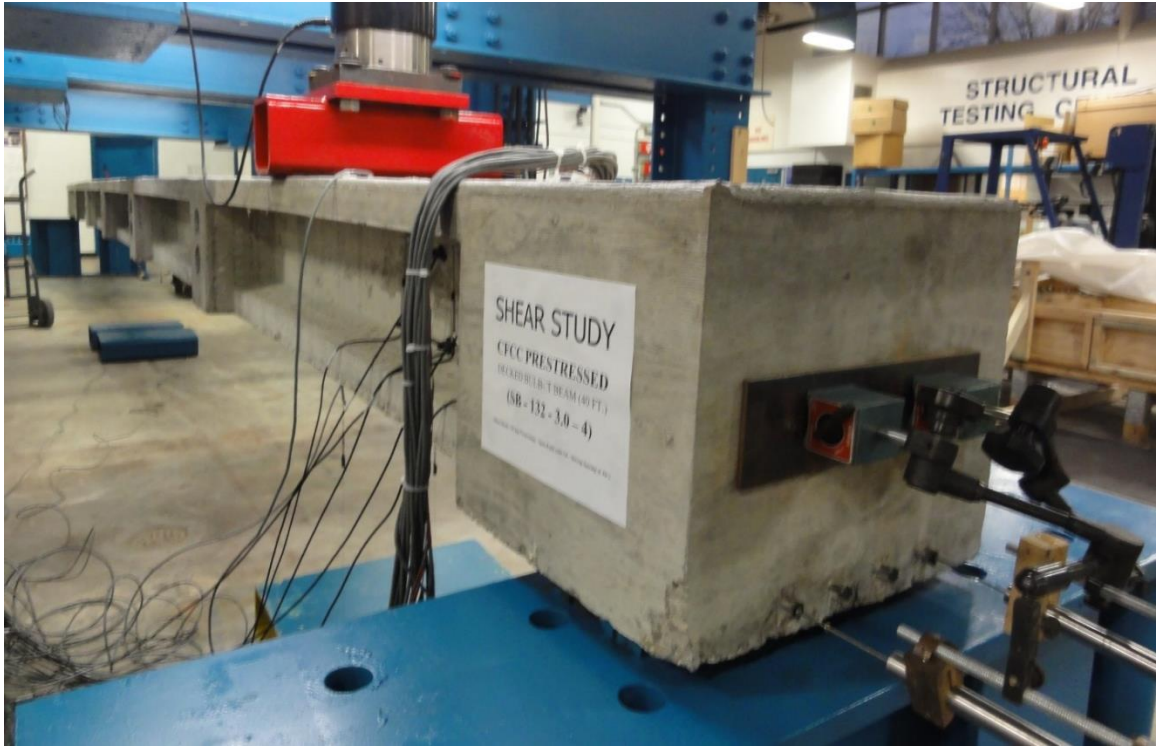
Figure 3.7-2 Monitoring slippage of prestressing CFCC strands using end LVDTs
