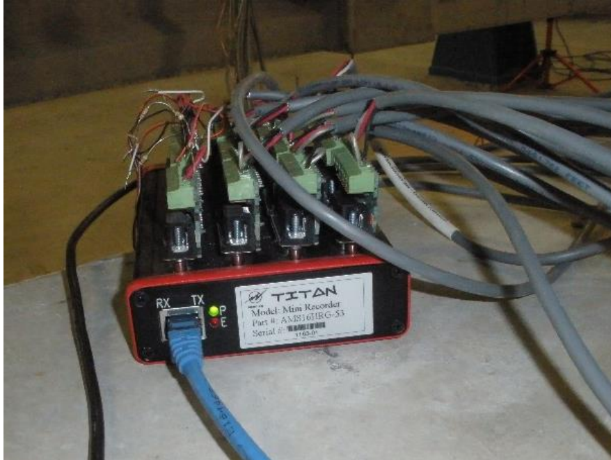
Figure 2.6-2 Mars Labs Titan model field pods for data acquisition
