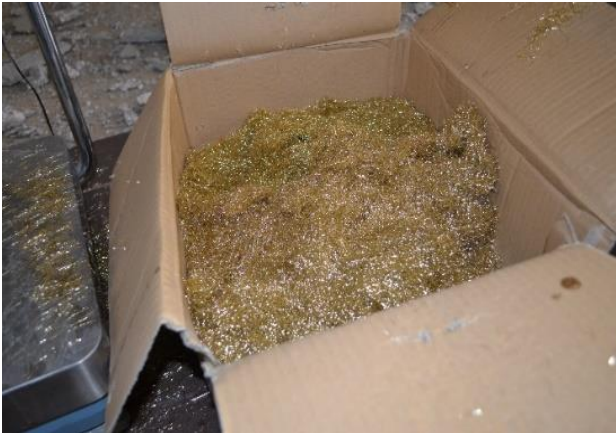
Coated steel fibers
