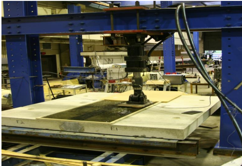
Figure 1.4-16 Testing of UHPC shear key joints between deck panels (Graybeal 2006)
