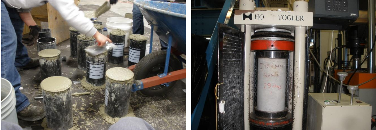
Figure 2.4-22 Concrete cylinders and uni-axial compression test
