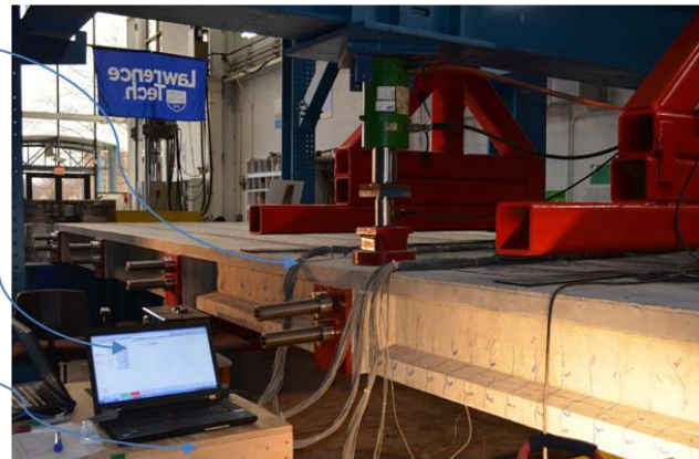
Figure 2.6-1 Data acquisition system wired into bridge model sensors
