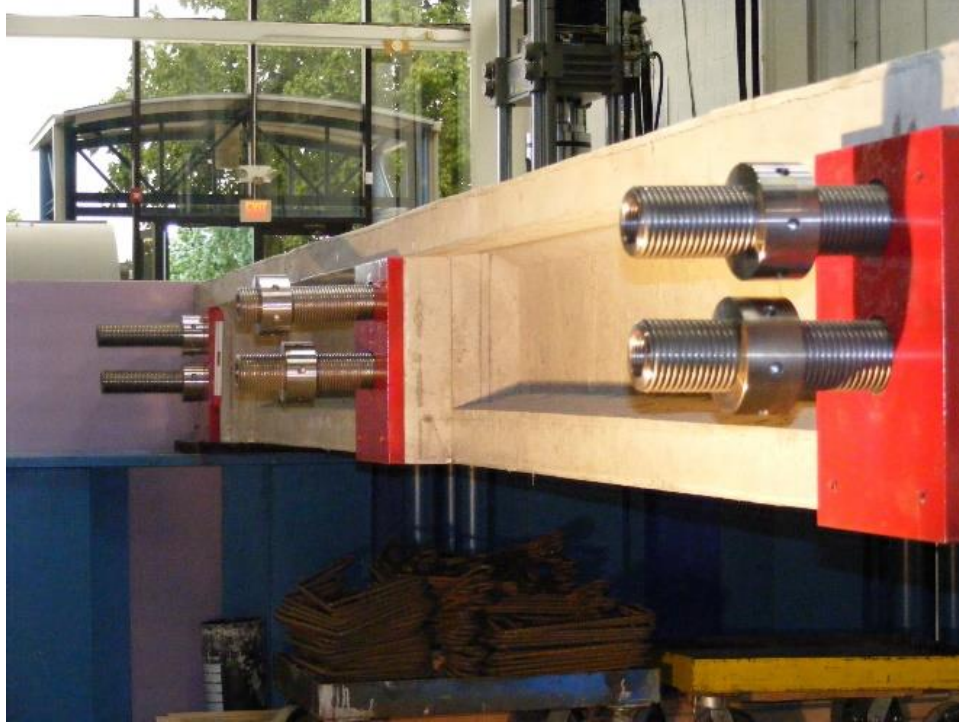
Figure 2.5-21 Transverse post-tensioning system with pre-attached sleeve-and-nut anchorage
