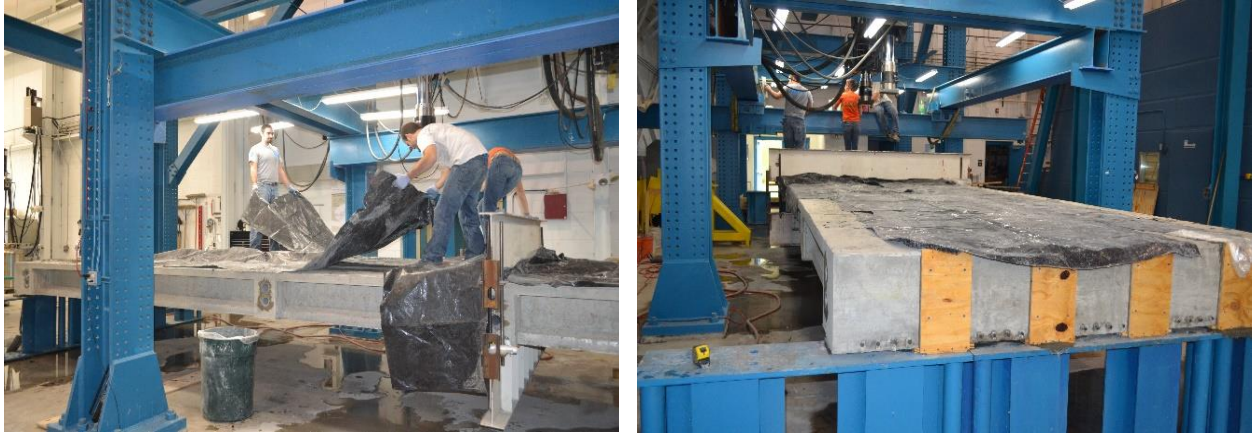
Figure 2.5-19 Curing of shear key joints using plastic sheets
