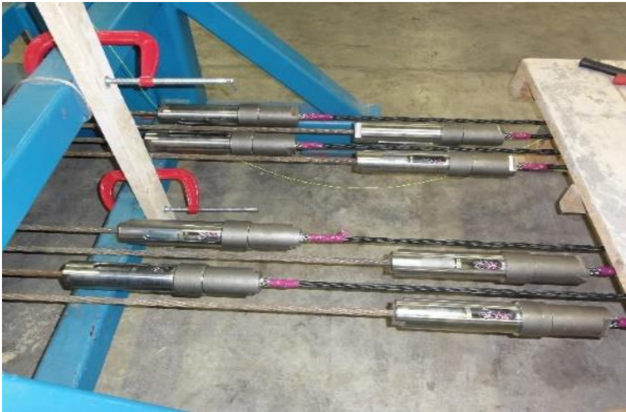
Figure 2.4-13 Completed coupler system for prestressing CFCC strands
