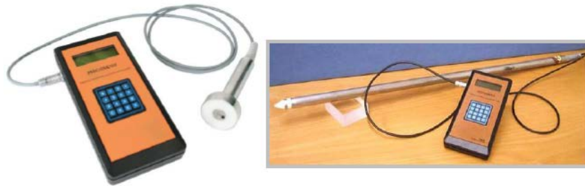
Figure B-5 Standard Adek Percometer™ with a surface probe and a tube probe [139]
