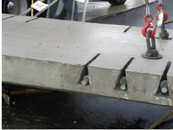
Figure 3-3 A narrow-mouth top surface slot system [10]
