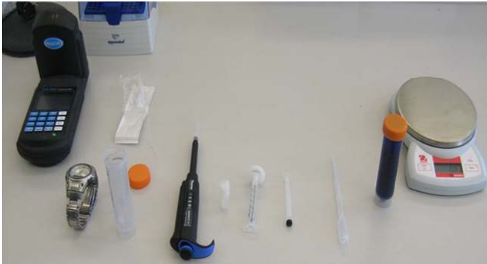
Figure B-1 Methylene Blue Test apparatus [139]
