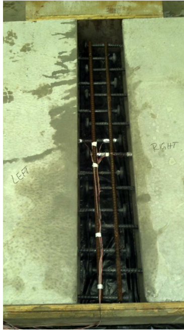
Figure 6.6: Strain gauge distribution on headed bar
