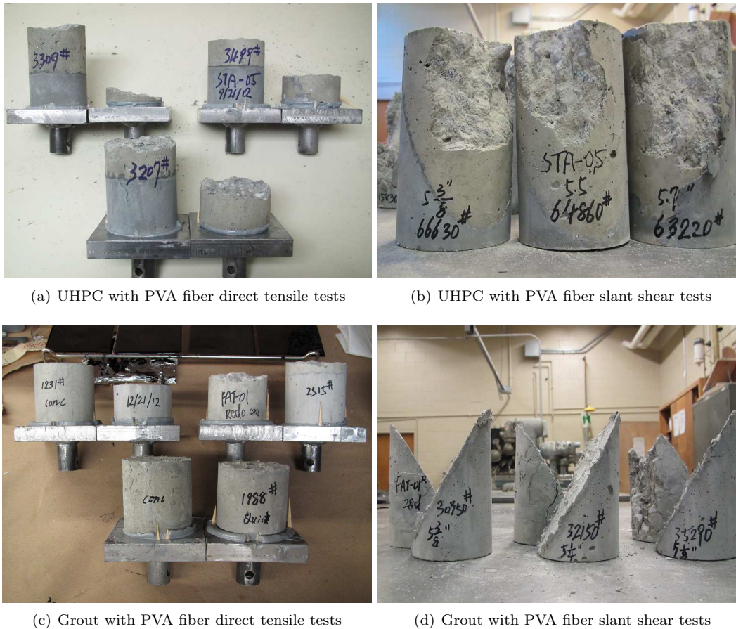
Figure 6.21: Cylinder failure modes in bond tests
