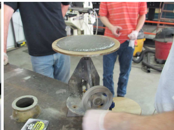
(b) Flow table test
