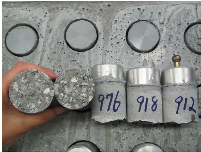
Figure 6.22: Pull-off test results for the UHPC with PVA combination
