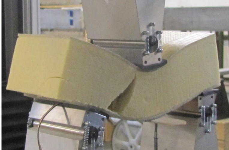
Figure 3.10: Ultimate Failure Due to Shear Failure of the Core Material for Type 1
