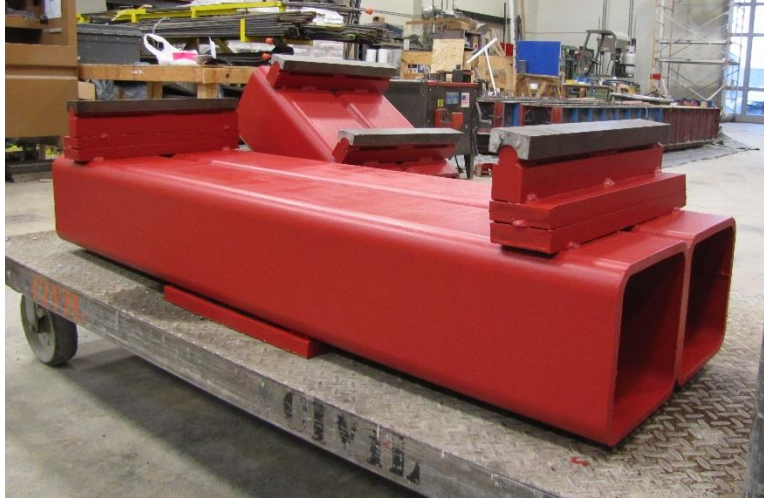
Figure 5.6: Fabricated Steel Test Fixture for Mid-Scale Panel Testing
