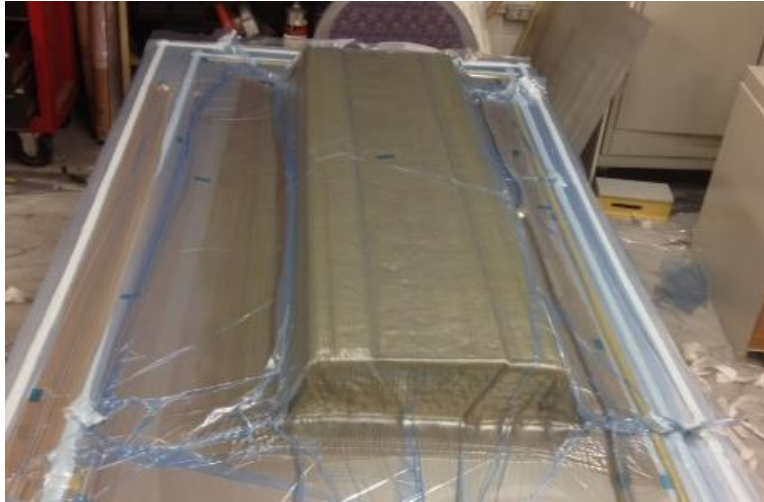
Figure 5.2: VARTM Manufacturing Process for Type 3 Mid-Scale Panels
