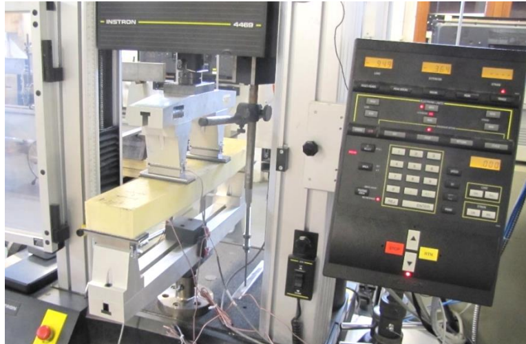
Figure 3.23: Four Point Flexural Test Setup
