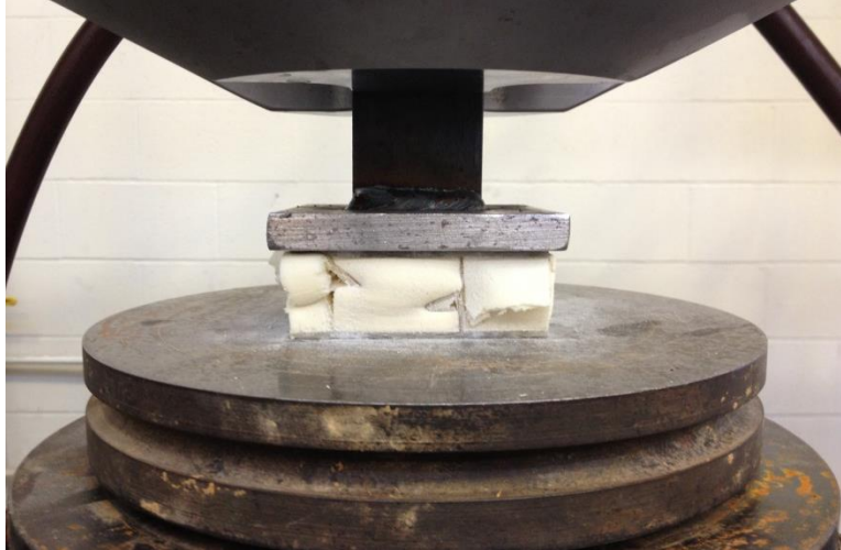
Figure 2.14: Damage at End of Test for Flatwise Compression Testing of Type 2
