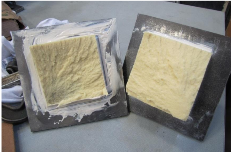
Figure 2.19: Fracture Surface for Flatwise Tension Testing of Type 1
