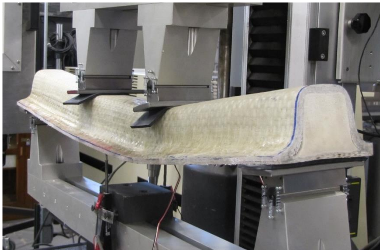
Figure 3.39: Ultimate Failure Due to Compressive Failure of the Top Facing for Type 3
