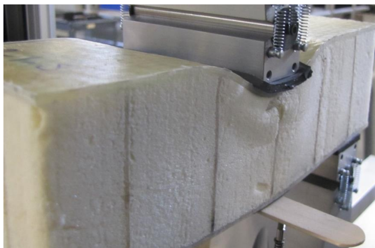
Figure 3.14: Ultimate Failure Due to Fracturing of Reinforcing Webs and Excessive Local Indentation for Type 2
