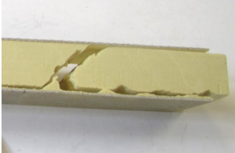
Figure 3.29: Ultimate Failure Due to Shear Failure of the Core Material for Type 1
