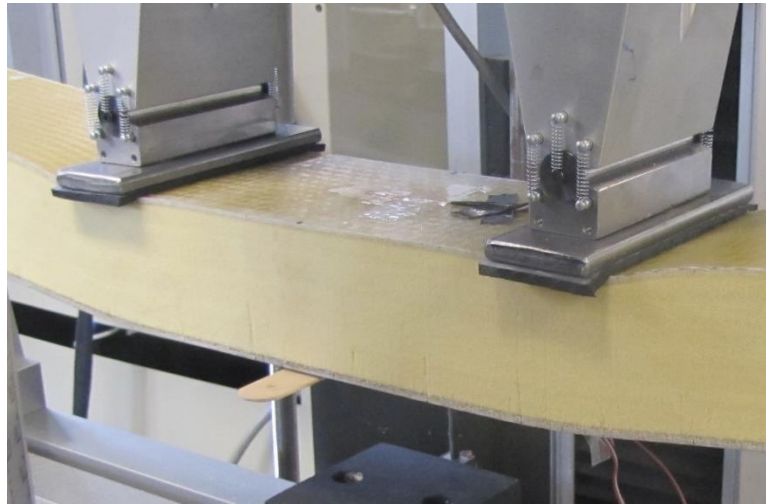
Figure 3.27: Initial Failure Due to Local Indentation for Type 1
