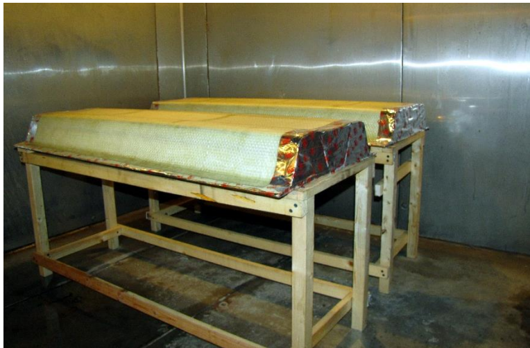
Figure 5.14: Durability Specimens within Environmental Chamber
