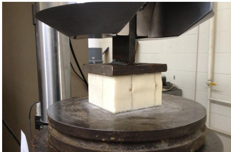
Figure 2.13: Damage at Failure for Flatwise Compression Testing of Type 2
