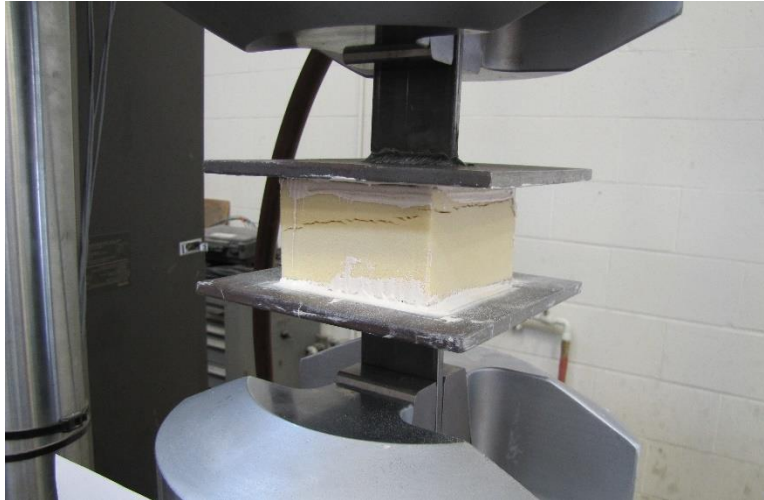
Figure 2.23: Damage at Failure for Flatwise Tension Testing of Type 3
