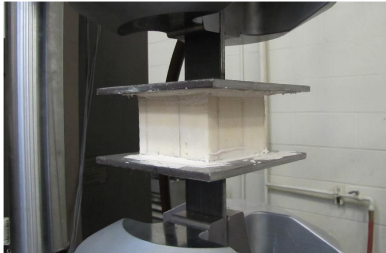
Figure 2.15: Prepared Specimen for Flatwise Tension Test
