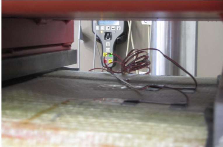
Figure 5.8: Strain Gauges Installed Along Top Facesheet at Mid-Span
