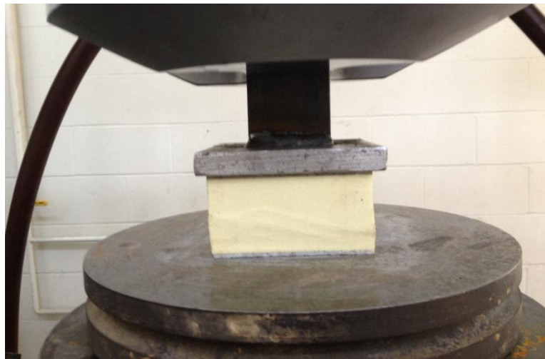
Figure 2.10: Damage at Failure for Flatwise Compression Testing of Type 1
