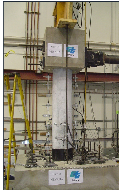
Figure 2.47 Segmental column model with rubber pad on a shake table at UNR
