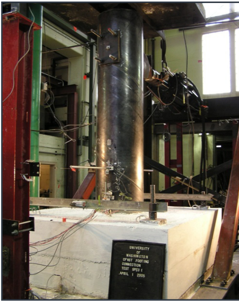
Figure 2.49 Concrete-filled steel tube column model tested at the University of Washington
