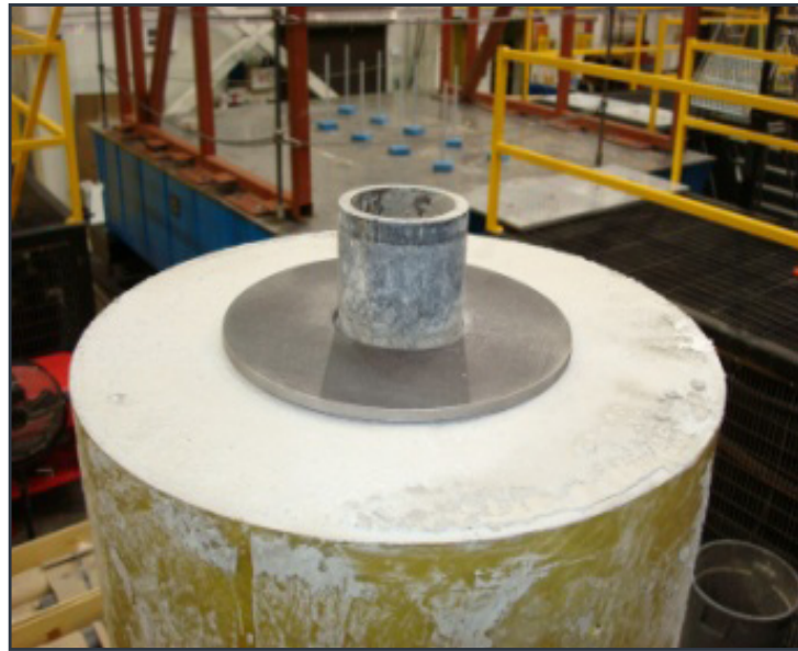
Figure 2.50 Steel pipe pin connection in a concrete-filled FRP tube column at UNR
