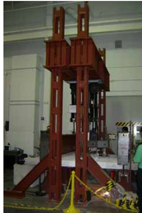
Figure 3.17. Apparatus Applying Fatigue Forces
