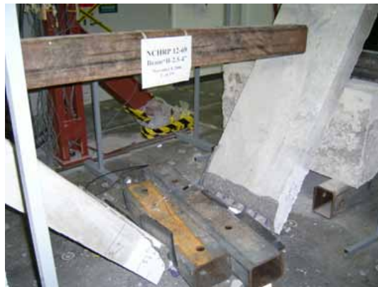
(b): Brittle Failure
