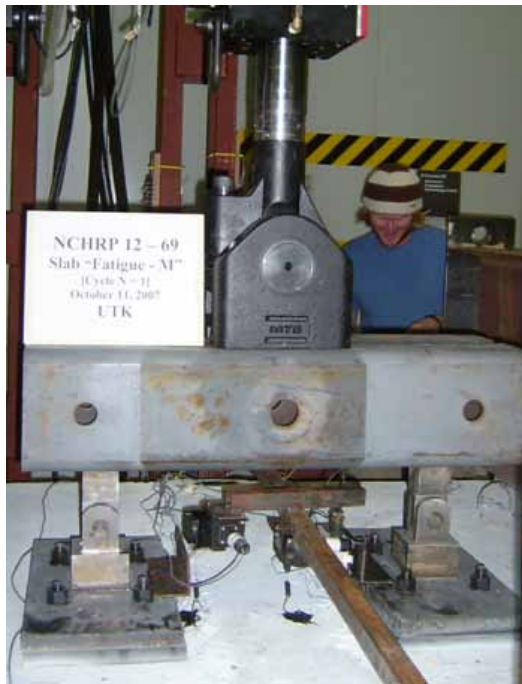
Figure 3.17. Apparatus Applying Fatigue Forces
