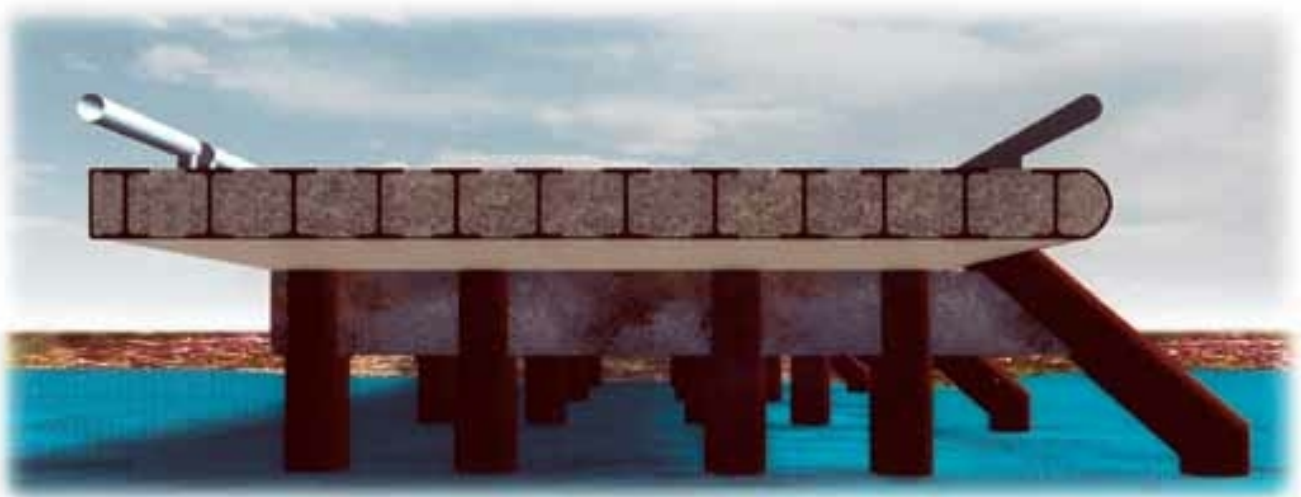
Cross-section conceptual drawing of a submersible bridge designed and fabricated for the North Slope of Alaska. See story on page 19.
