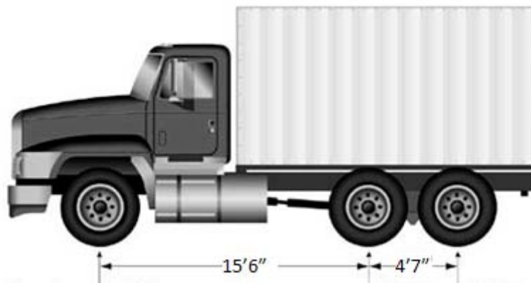
Figure 6-9. Truck type II configuration
