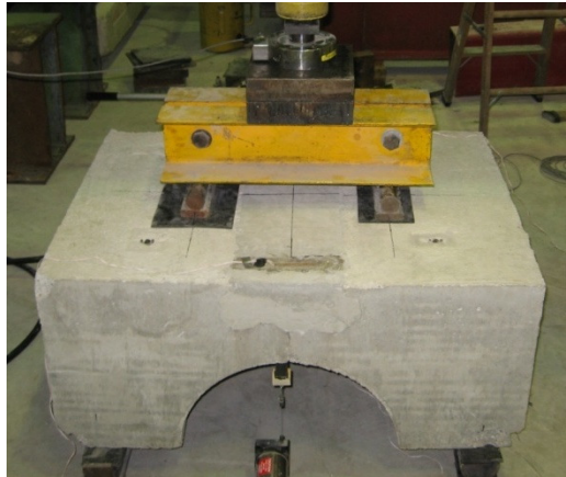
b) Photograph of ultimate load test
