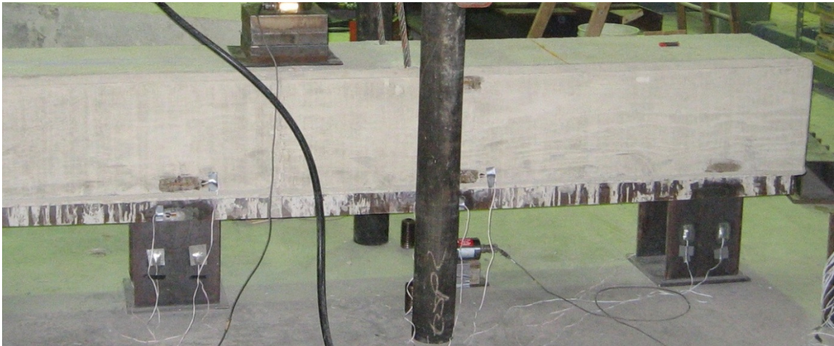
b) Cap 2 fabricated with W12x26
