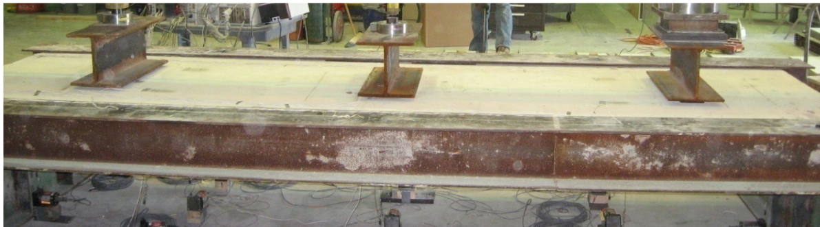
b) Photograph of backwall with HP 10's on edges
