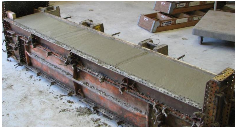
Figure 19. Finished concrete surface of Type 1 Connection.
