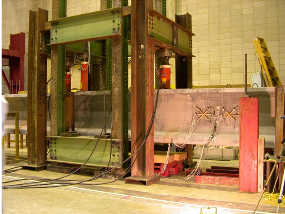
Figure 9. Shear Test Setup.
