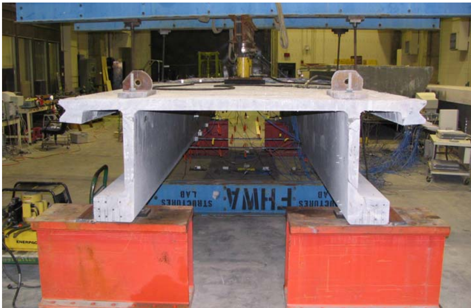
Figure 16. Transverse deck test of first generation pi-girder at Turner Fairbank Laboratory (Photo courtesy of FHWA)
