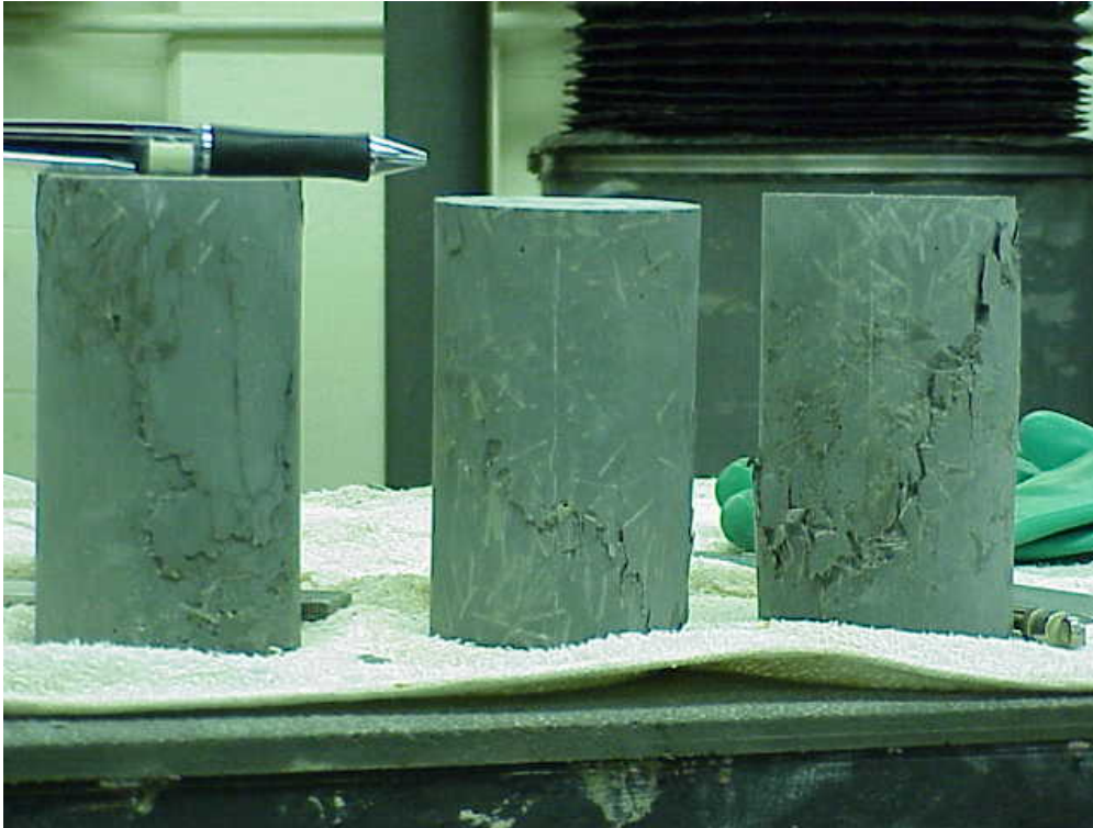
Figure 2. Broken Test Cylinders
