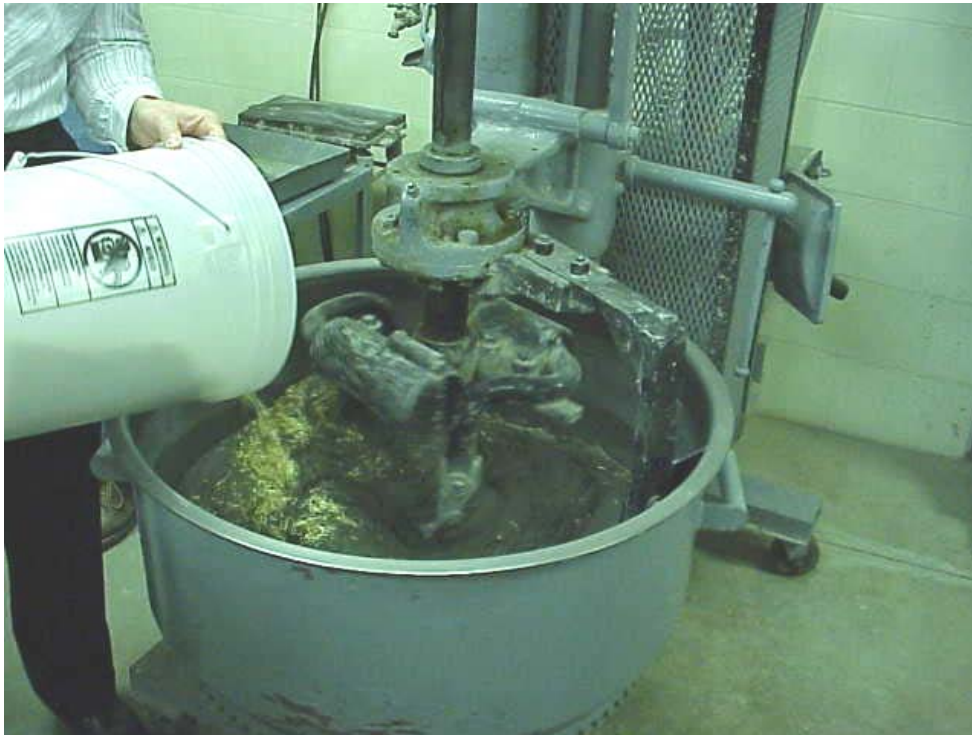
Figure 1. Mixing of UHPC in the Materials Laboratory of Iowa DOT
