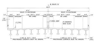
Figure 3. Superstructure cross section.
