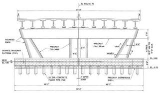
Figure 6. Final precast pier configuration.
