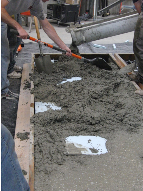
Figure 14: Placing Concrete in Shear Specimen.
