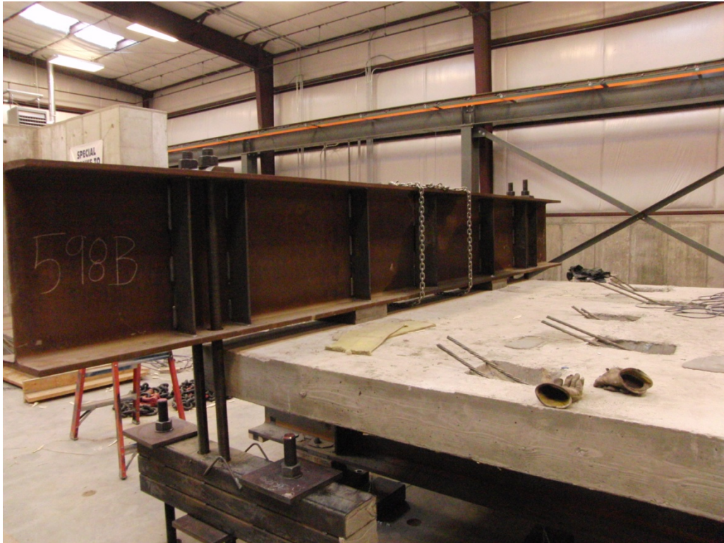
Figure 28: Uplift Restraint Beam.
