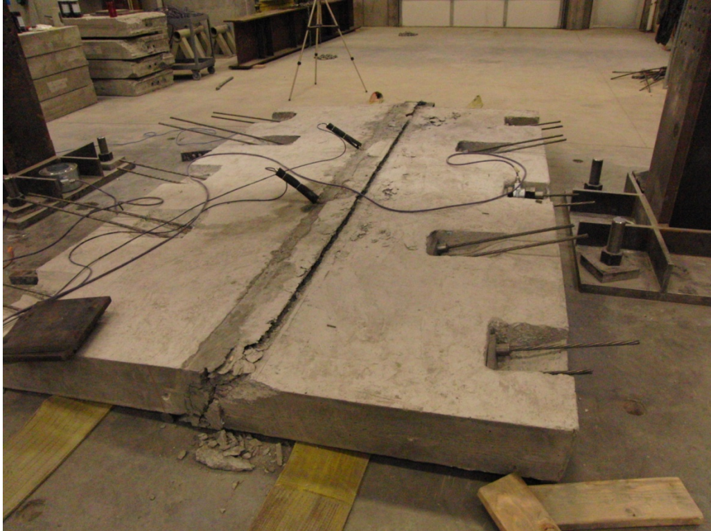
Figure 26: Shear Crack Propagating Along Joint.
