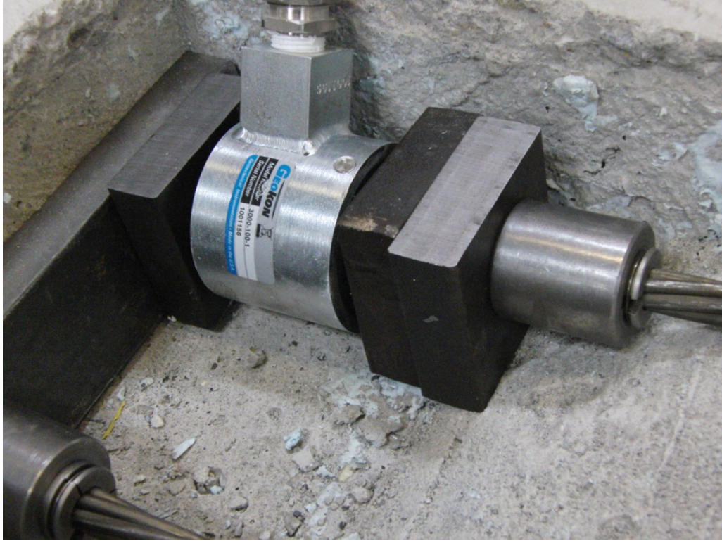
Figure 18: Load Cell on Curved Strand Connection.
