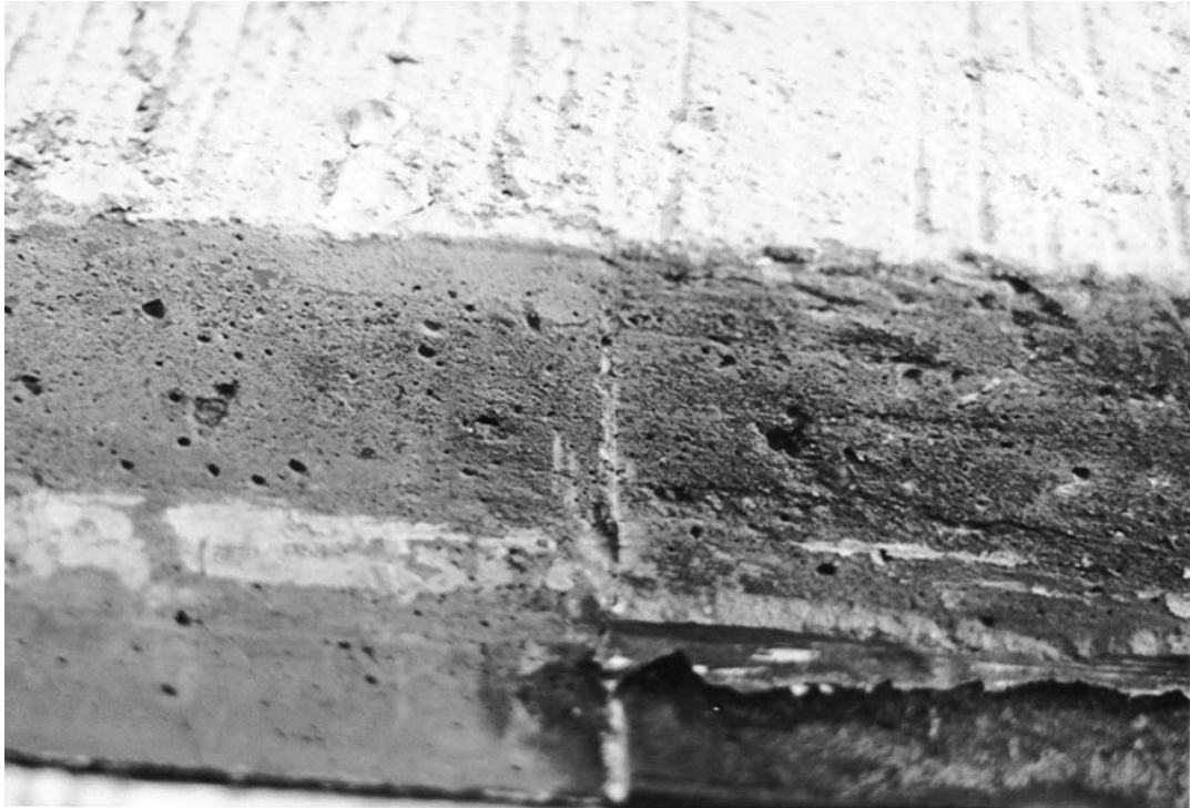
Figure 65. Bar/Plate Connection after Cyclic Loading.
