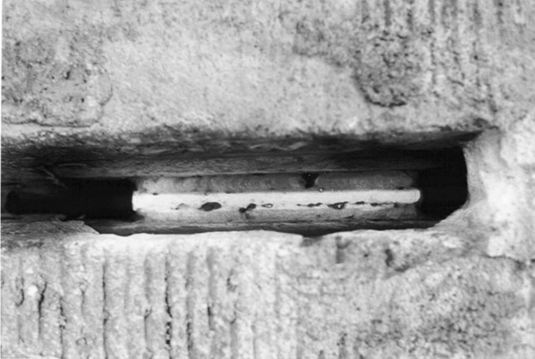
Figure 65. Bar/Plate Connection after Cyclic Loading.
