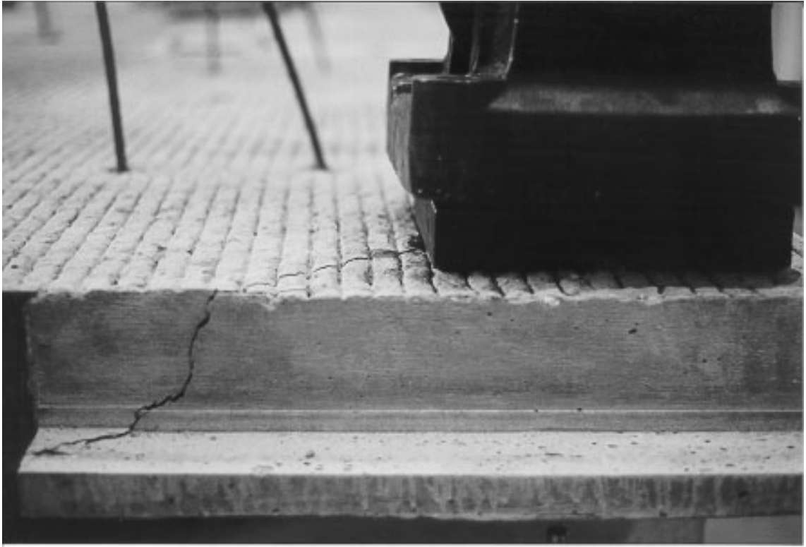
Figure 38. Failed Flange from Loading Outside Flange Edge.
