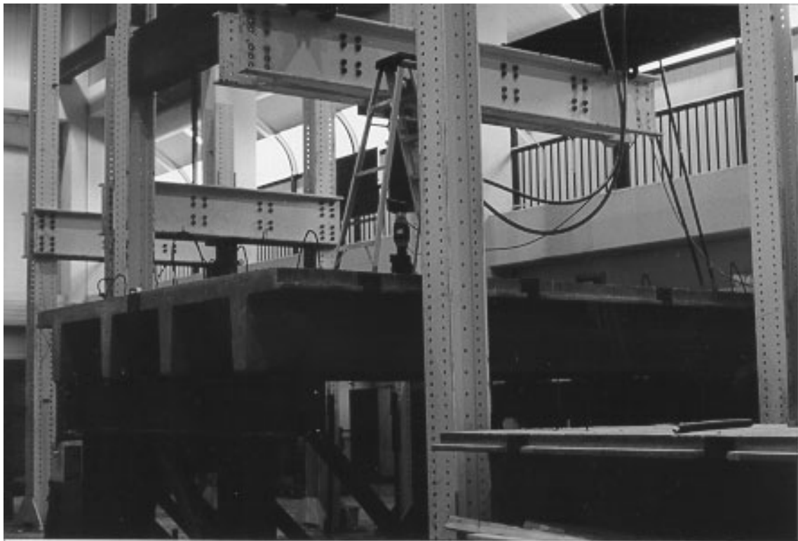
Figure 31. Double Tee Laboratory Bridge.
