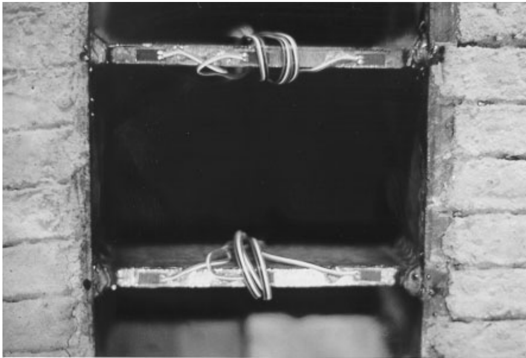
Figure 32 (b). Strain Gages on Connection Plates.
