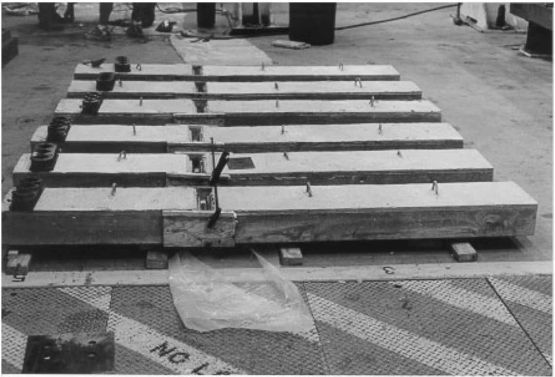
Figure 41. "Simple" Connection Test Specimens.
