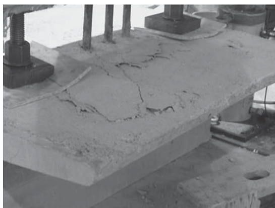
(b) Top surface cracks at failure
