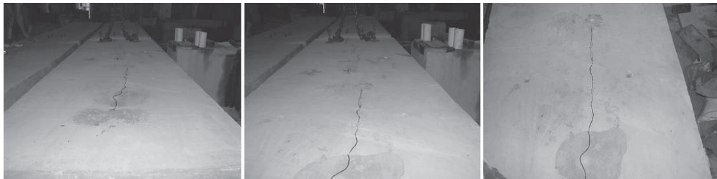
Beam #2 (4-ft stud cluster spacing)
