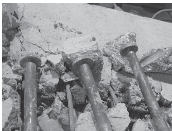
(d) Studs after being pulled away from the specimen
