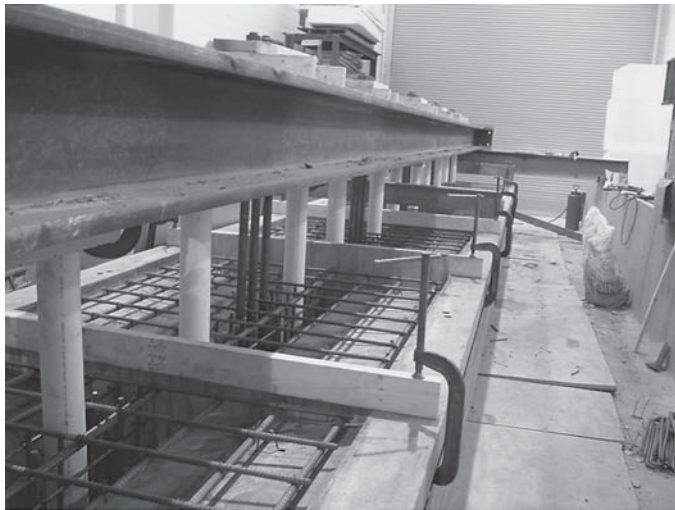
(a) The test specimens ready to receive concrete
