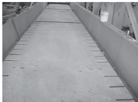
Figure 45. Panel P1, P2, and P3 after 7 days of moist curing.
