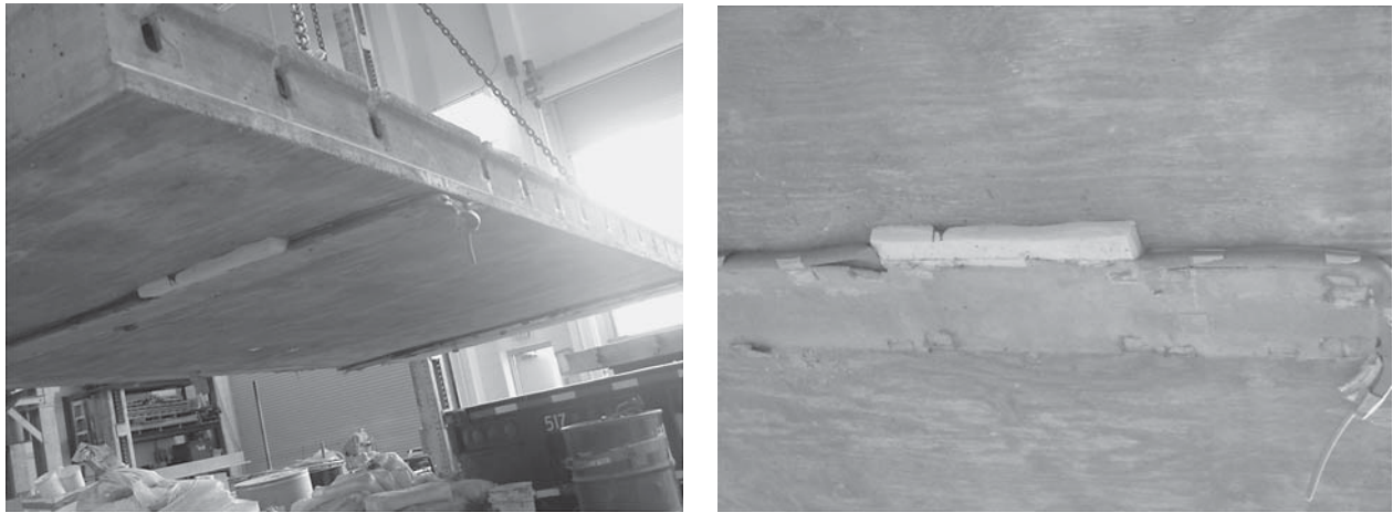
(a) The Haunch fully filled with Grout with no Air Voids
