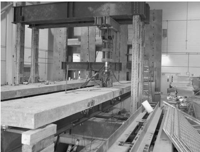
Figure 88. Fatigue test setup.
