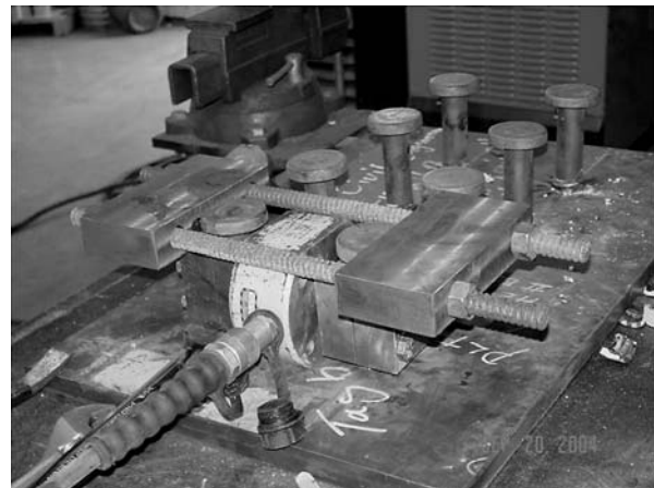
Figure 75. Welding of the 1/4-in. studs and the quality control tests.
