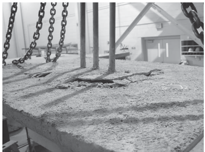
(b) Top surface cracks at failure
