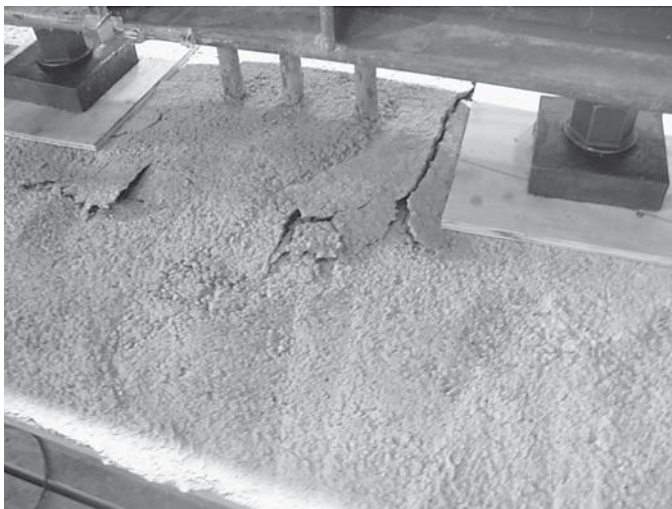
(b) Top surface cracks at failure
