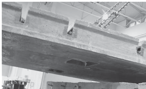
Figure 45. Panel P1, P2, and P3 after 7 days of moist curing.
