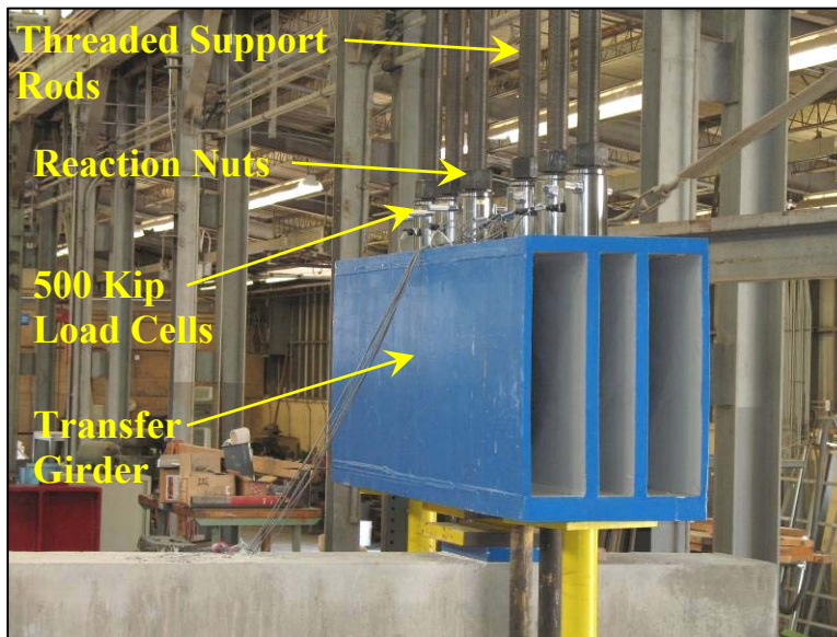
Figure 3.27: Load cells measure the reaction in each rod.
