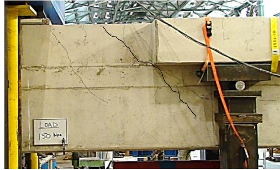
SL3-42-1.85-03: first crack at 30% ultimate load
