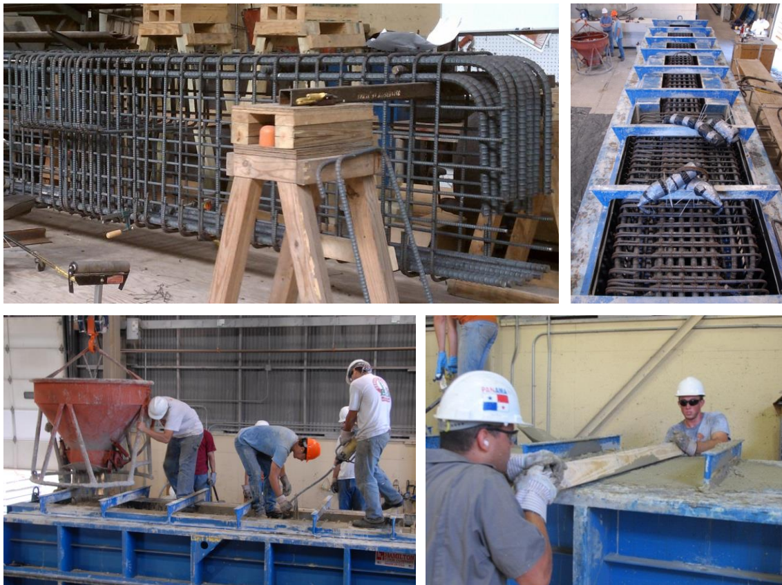
Figure 3-17: Fabrication of specimens
