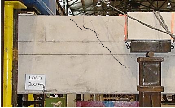
SL3-42-1.85-03: first crack at 30% ultimate load
