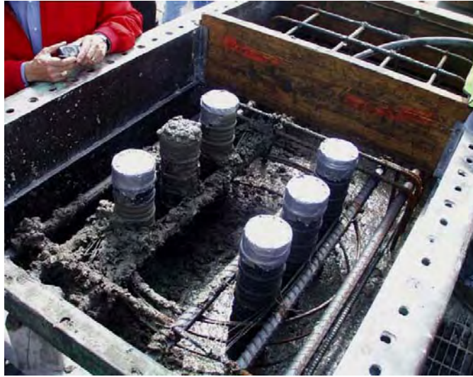
Figure 2-1: Corrugated ducts and joint reinforcement (Brenes 2006)
