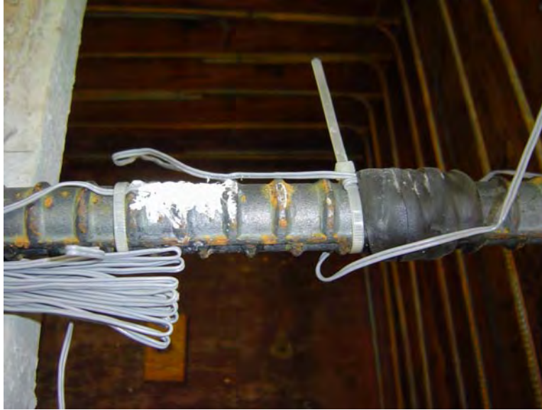
Figure B-24: Strain gage coated with M-Coat (left) and fully protected (right)
