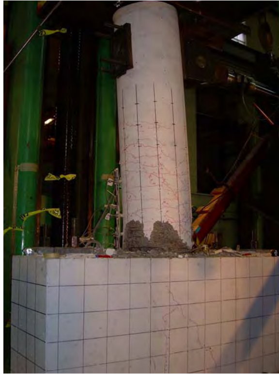
Figure 4-41: Specimen LB8-D1 displaced during Cycle 34 (7.20%/-7.06%)
