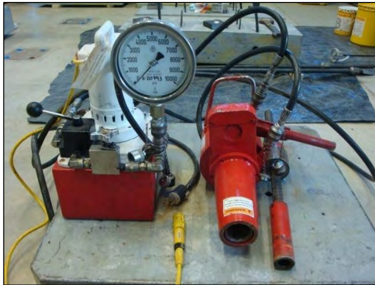
Figure 38: DSI's post tensioning stressing equipment
