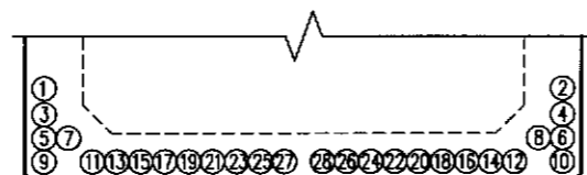
DETENSIONING PROCEDURE - B33x48
