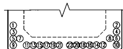
DETENSIONING PROCEDURE - B33x36
