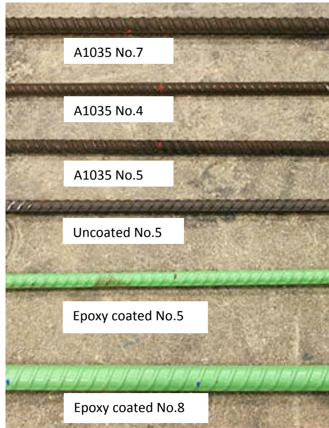
Figure 2. Photo. Reinforcing bar rib pattern.
