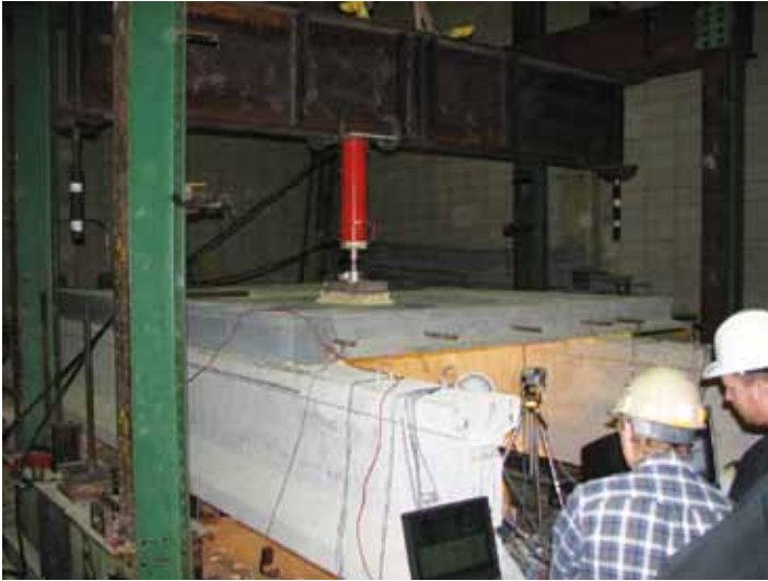
Figure 18 - Load testing of the waffle slab at ISU's Structural Engineering Laboratory; deck panel service, fatigue and strength level tests were performed; a similar series of tests were also performed to assess the panel-to-panel transverse joint performance
