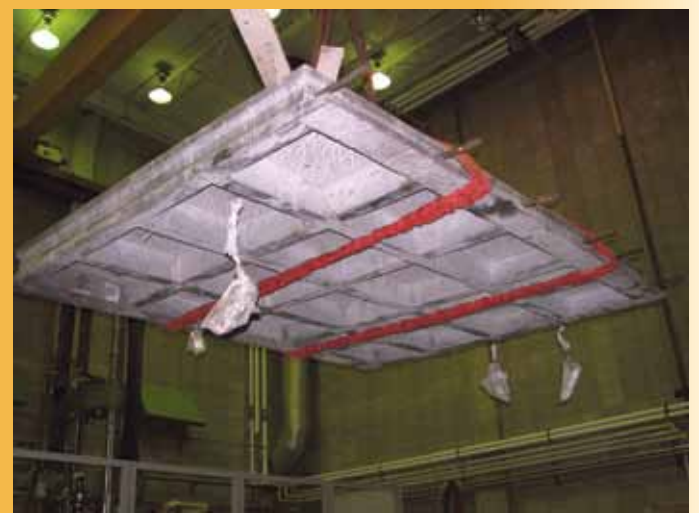
Waffle slab placement for laboratory testing after shipment from Coreslab Structures Inc.
