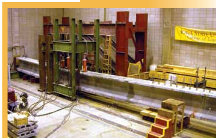
Laboratory loading test setup evaluates flexural/shear characteristics of a full-scale beam.
