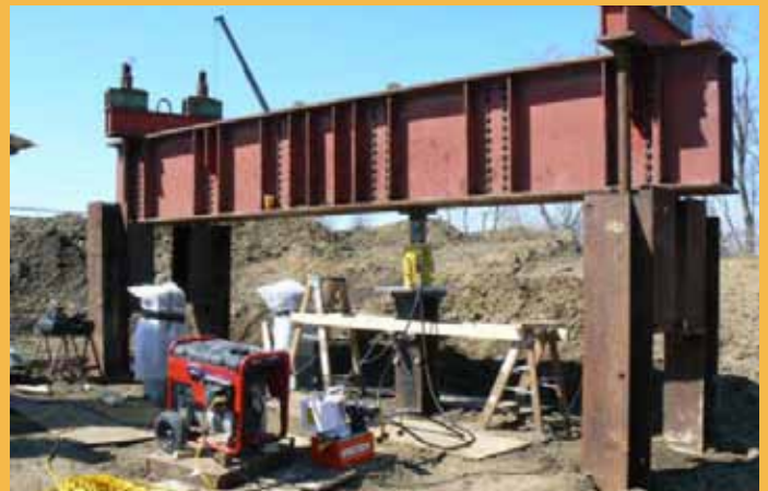
Vertical load test of the steel pile at the Oskaloosa test site
