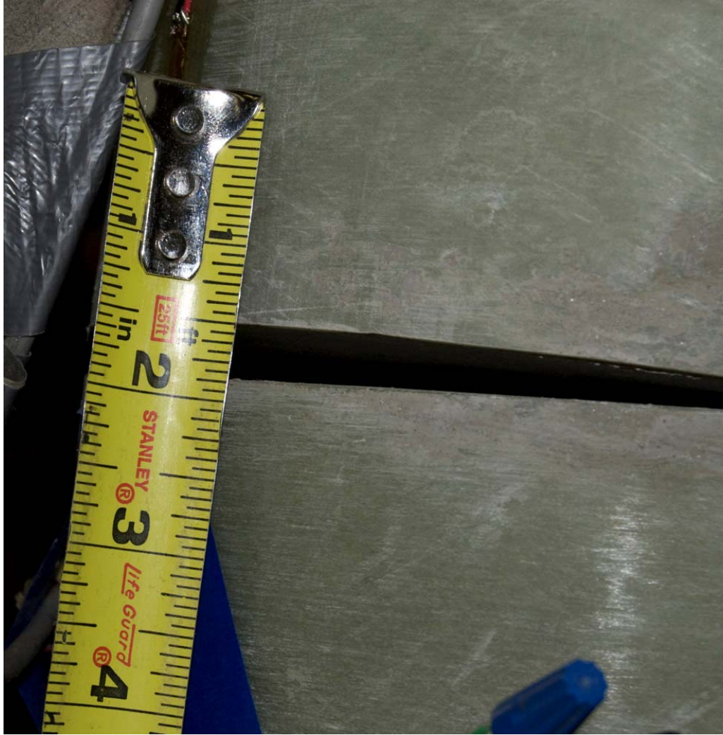
Figure 18: Specimen FRP-S Rocking Gap Between Segments 1 & 2
