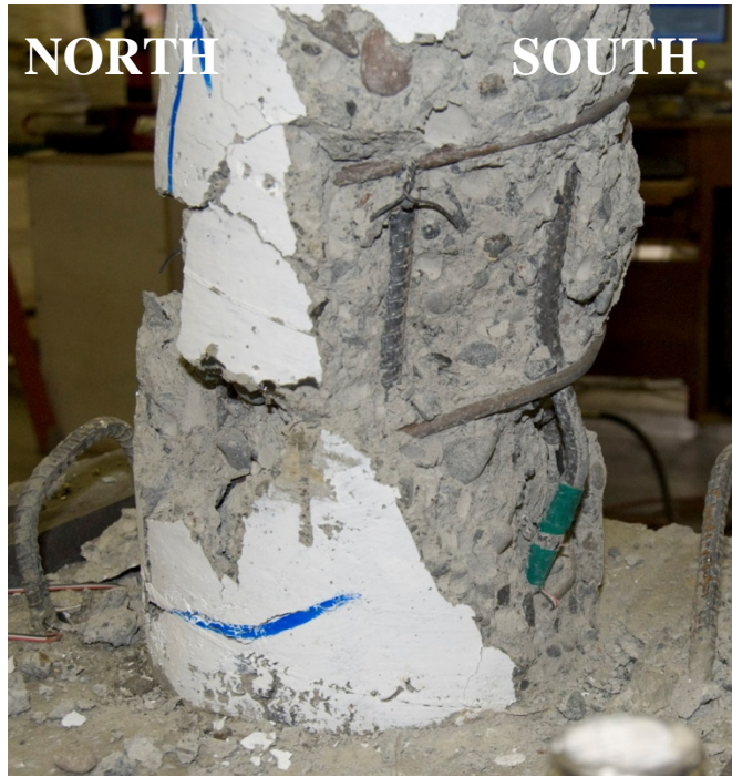
Figure 11: Specimen RC Longitudinal Rebar Buckling After Testing
