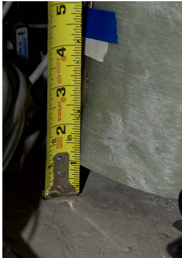
Figure 17: Specimen FRP-S Rocking Gap Between Base & Segment 1
