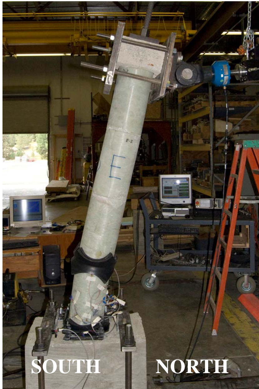
Figure 24: Specimen FRP-R Under Displacement
