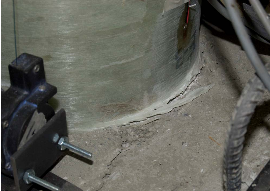
Figure 20: Specimen FRP-S Damage to FRP
