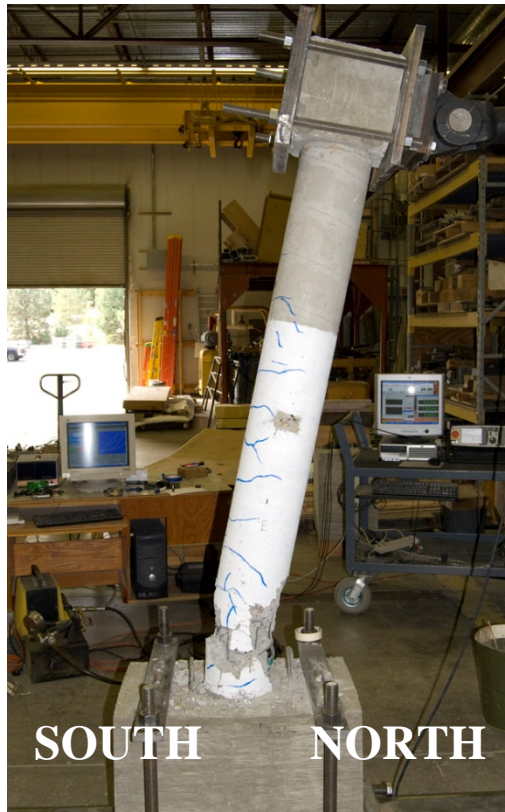
Figure 12: Specimen RC at 10 in. Displacement
