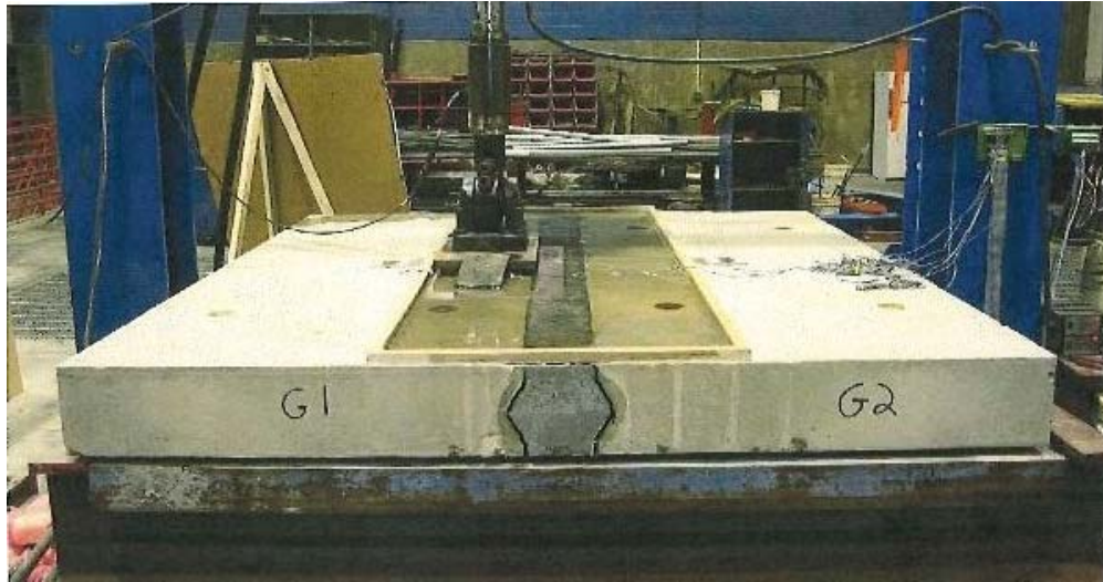
Photo 1 Precast Prestressed HPC Deck Panel Joint – FHWA Cyclic Testing 1
