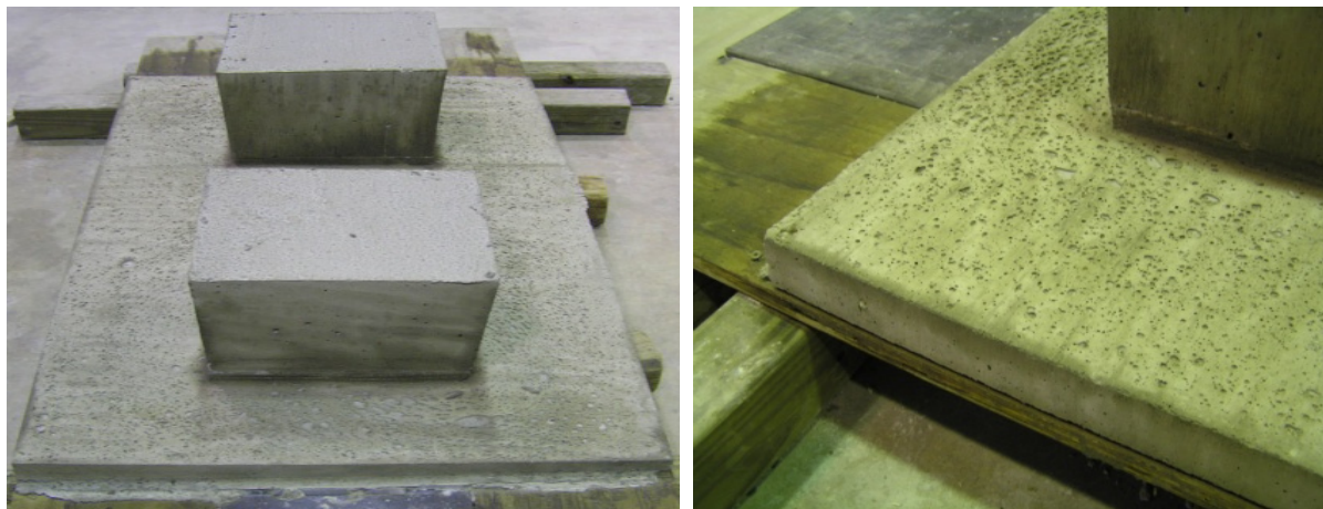
a. Grout filled pockets and haunch
