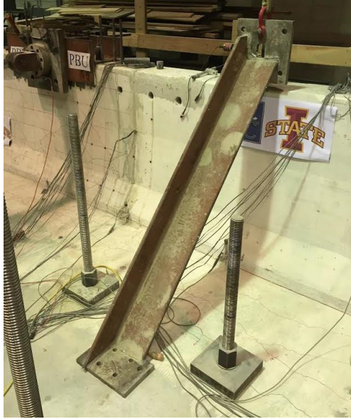
Figure 22 Beam used to brace the u-bar connected barrier during Test 4
