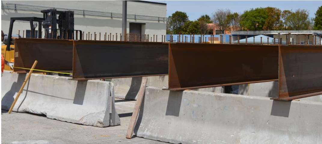
Fig. 2. Laboratory test specimens under construction, showing the girders and Nelson studs.
