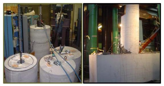
Figure 3: UW Test setups of large bar-duct pullout and column-to-cap-connection
