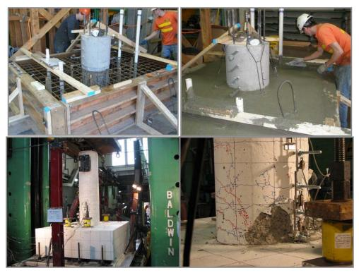
Figure 6: UW Test setups for precast column-to-footing connection
