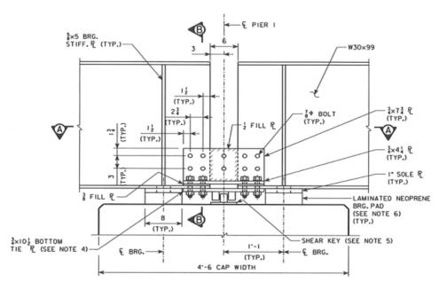
Figure 9. Structural steel connection between adjacent spans
