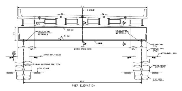
Figure 5. Typical section through pier
