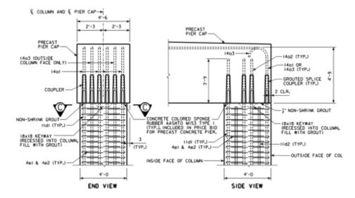
Figure 7. Connection of precast cap to precast column
