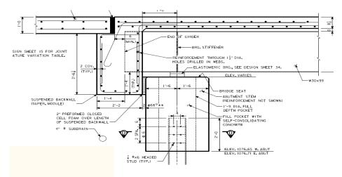
Figure 4. Precast abutment with suspended backwall
