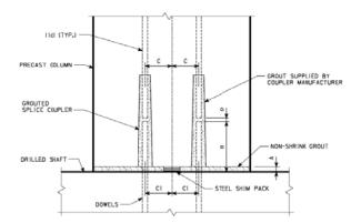
Figure 6. Grouted splice coupler details
