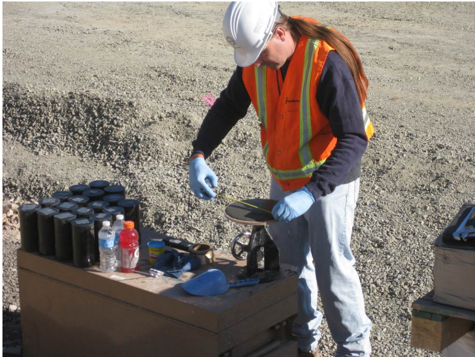
Figure 50. Measuring the flow using ASTM C1437—Standard Test Method for Flow of Hydraulic Cement Mortar.
