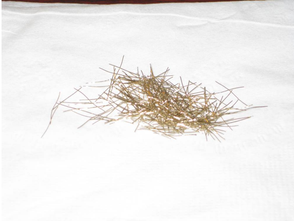
Figure 49. Close-up view of UHPC fiber.
