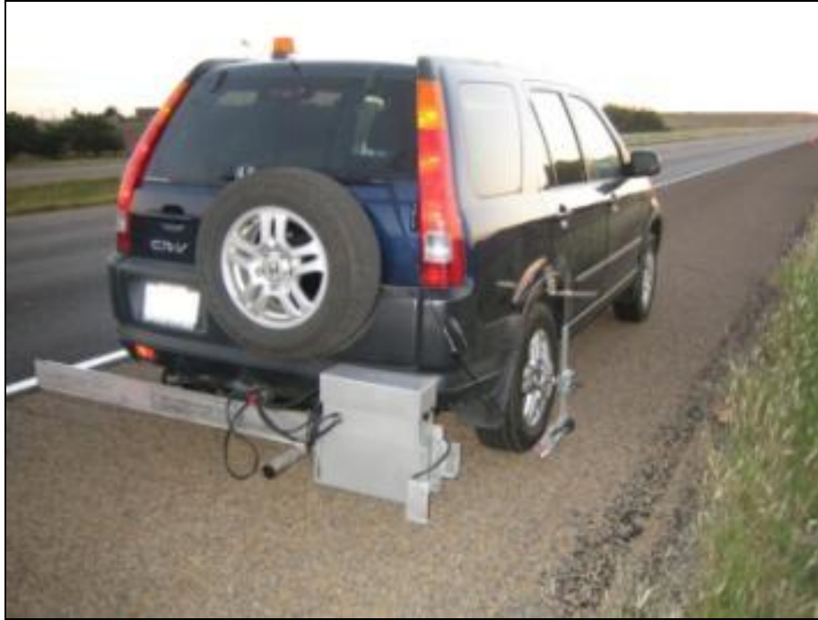
Figure 63. High-speed inertial profiler mounted behind the test vehicle.
