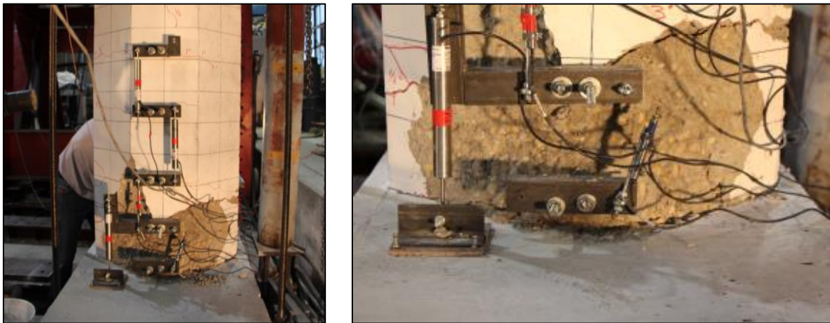
Figure 4-56. Damage state for FGSS-CIP at 6% drift ratio: cracks and spalling, yield penetration.
