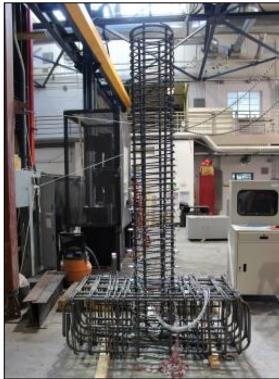
(b) Rebar cage ready to cast concrete.
