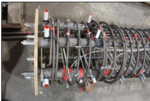
(a) Column end GGSS and overlapping spiral. (b) Footing dowel bars tied to rebar cage.
