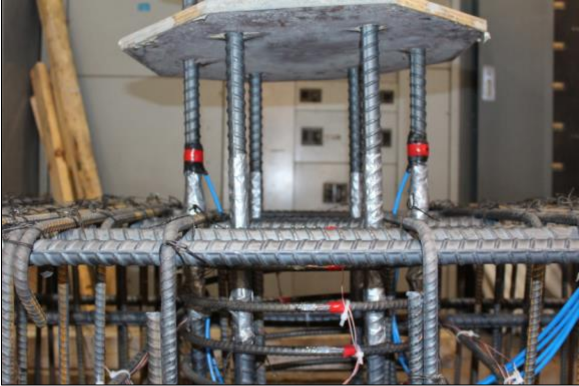
Figure 2-16. Debonded region of the dowel bars for GGSS-3.
