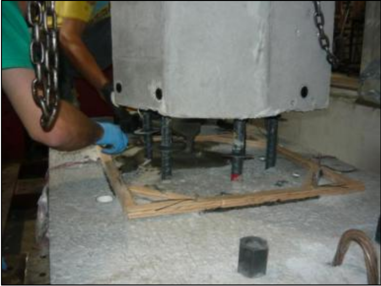
Figure 2-7. Grouting operation for GGSS-1.
