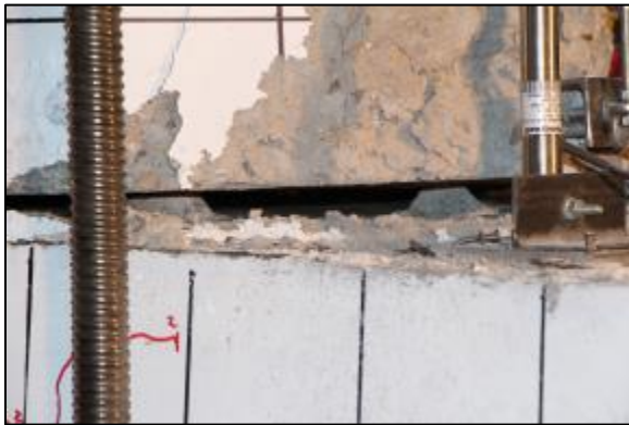
(c) Bar pull-out during 6% drift ratio.
