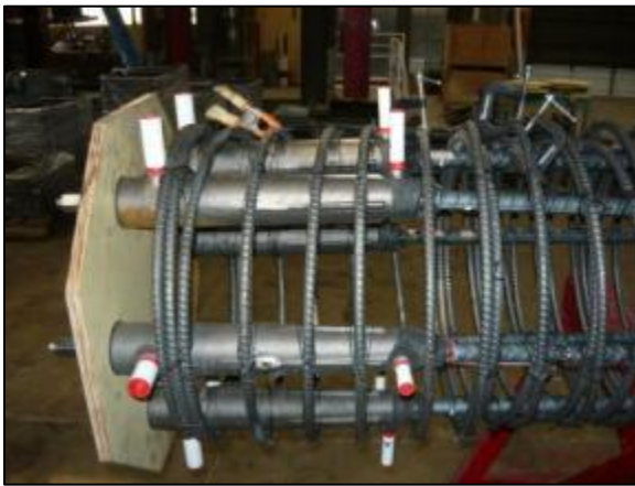
(a) Column end GGSS and overlapping spiral. (b) Footing dowel bars with inward tails.
