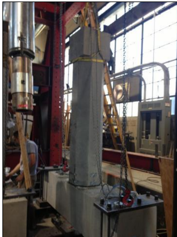
Figure 2-45. FGSS-3 in the final position.
