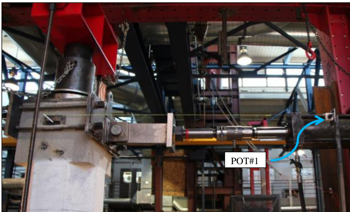
Figure 3-4. String potentiometer on west side of specimen GGSS-3.
