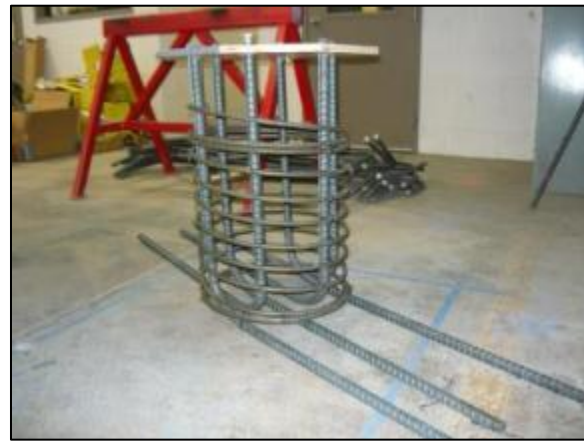
(a) Column end GGSS and overlapping spiral. (b) Footing dowel bars with inward tails.
