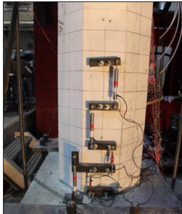
(b) LVDTs attached to fixture.
