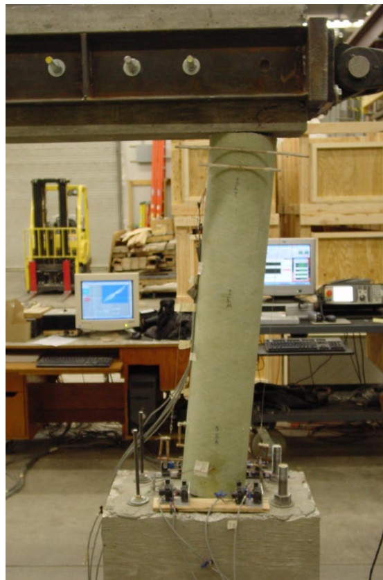
Figure 5.2.13: Northern column of specimen F-FRP1 undergoing rocking mechanism
