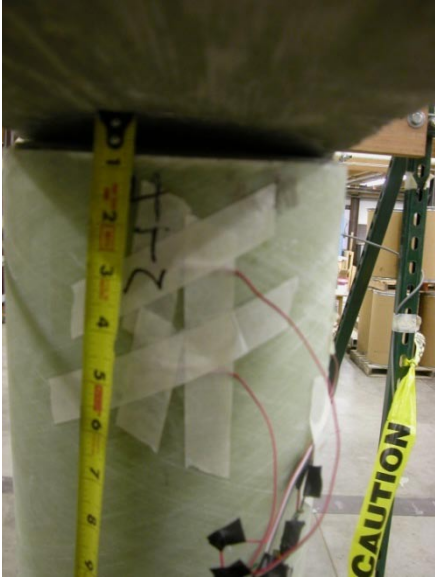
(b) Gap at column-beam interface of southern column
