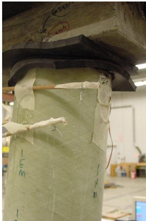
Figure 5.2.24: Upper column segment of the northern column of specimen F-FRP3-R at maximum displacement
