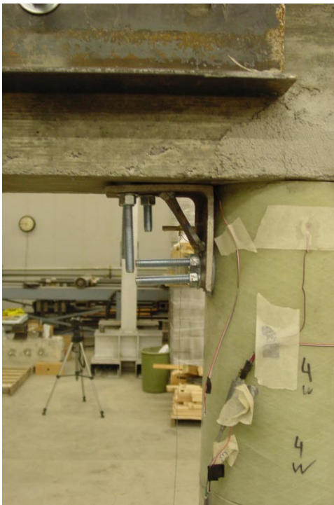
Figure 3.1.15: Energy dissipating device attached to southern column of specimen F-FRP3-S
