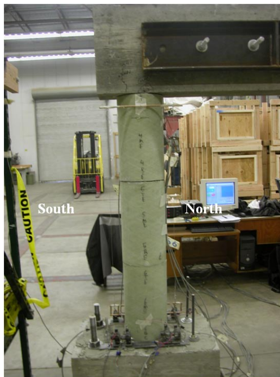
Figure 3.1.8: Southern column of specimen F-FRP3 prior to testing
