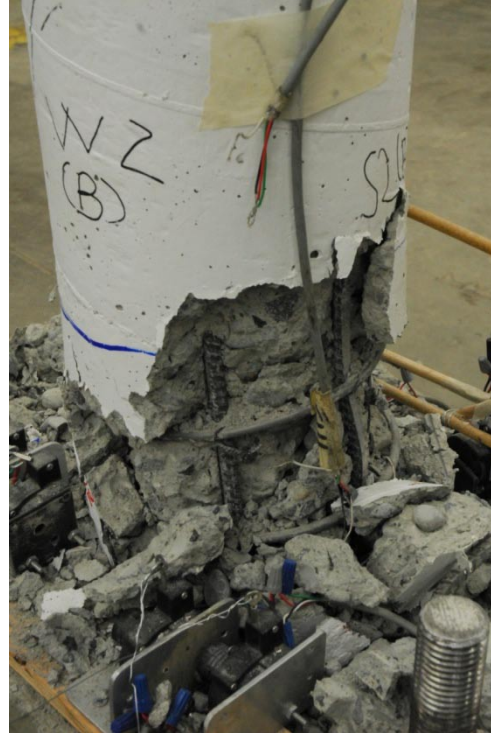
Figure 5.2.6: Core concrete crushing at 3.6 in. displacement
