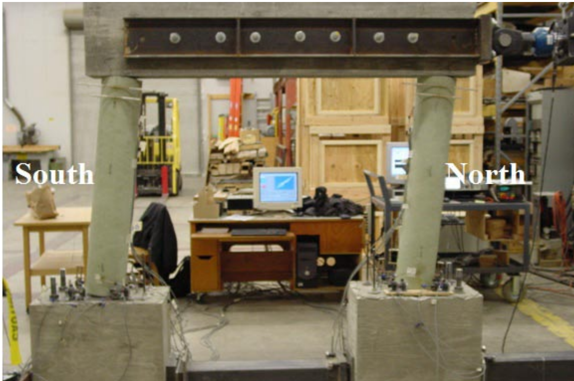
Figure 5.2.10: Specimen F-FRP1 at the end of the test
