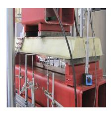
Polyurethane Foam Infill for Fiber-Reinforced Polymer (FRP) Bridge Deck Panels
