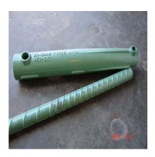
Evaluation of Grout-Filled Mechanical Splices for Precast Concrete Construction
