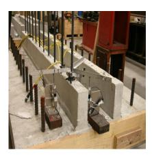
Bond Behavior of Reinforcing Steel in Ultra-High Performance Concrete
