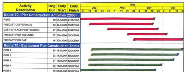
**Figure 16. Construction schedules for the eastbound precast pier operations and the durations of Piers 1EB through 5EB.**
