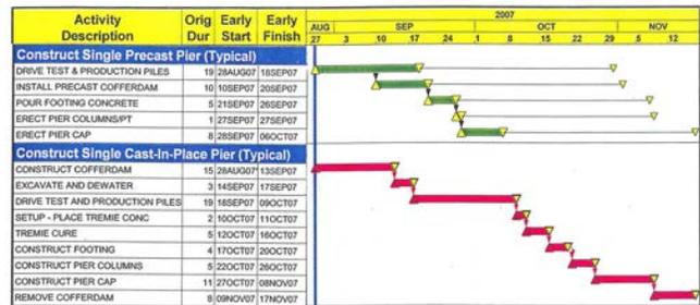
**Figure 18. Construction schedules for a typical cast-in-place pier and an optimized precast pier.**
