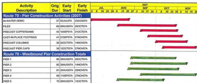
**Figure 17. Construction schedules for the westbound precast pier operations and the durations of Piers 1WB through 5WB.**
