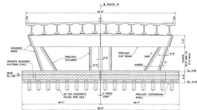
**Figure 6. Final precast pier configuration.**
