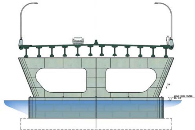
**Figure 5. Initial architectural recommendation for the proposed piers.**
