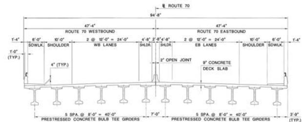
**Figure 3. Superstructure cross section.**
