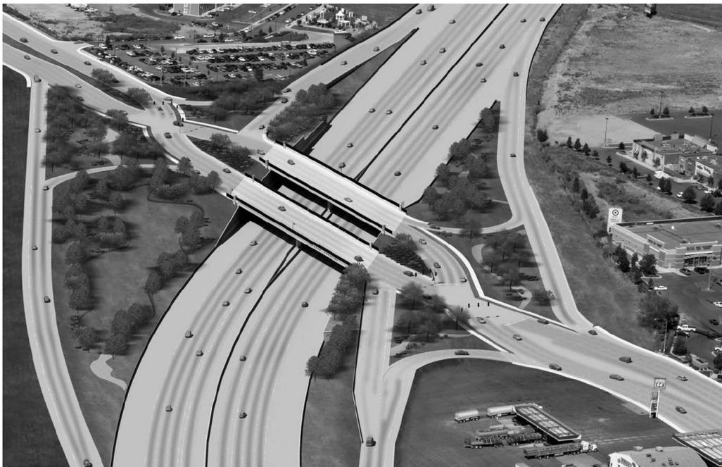
Figure 1 – Diverging Diamond Interchange Rendering
